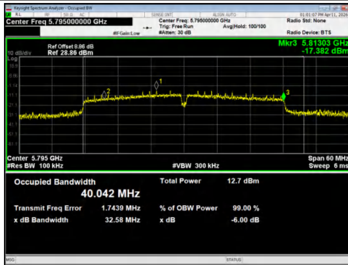
-6dB Bandwidth NVNT ac80 5775MHz Ant1
