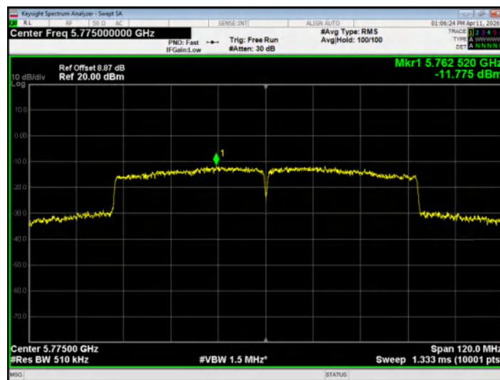
PSD NVNT n20 5745MHz Ant1
