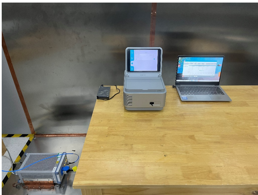
Photograph 3: Set-up photo for AC Conducted Emissions
