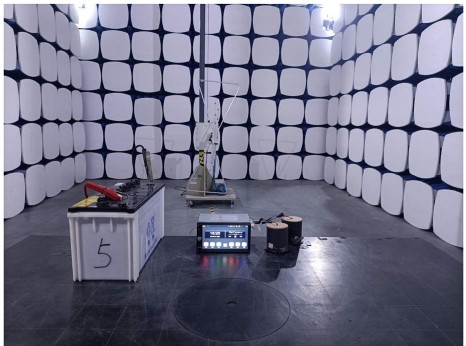
Radiation Emission Test Setup (30MHz to 1GHz)
