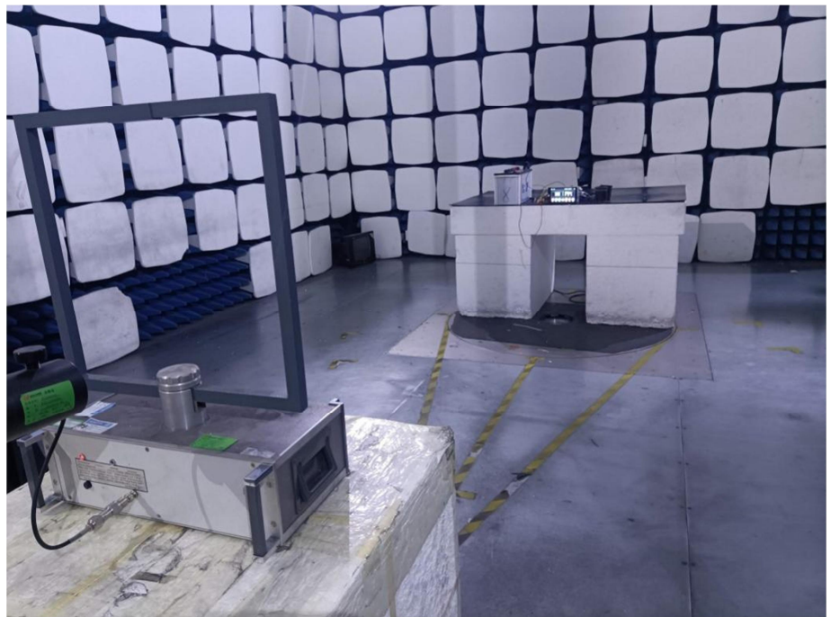
Radiation Emission Test Setup (Below 30MHz)
