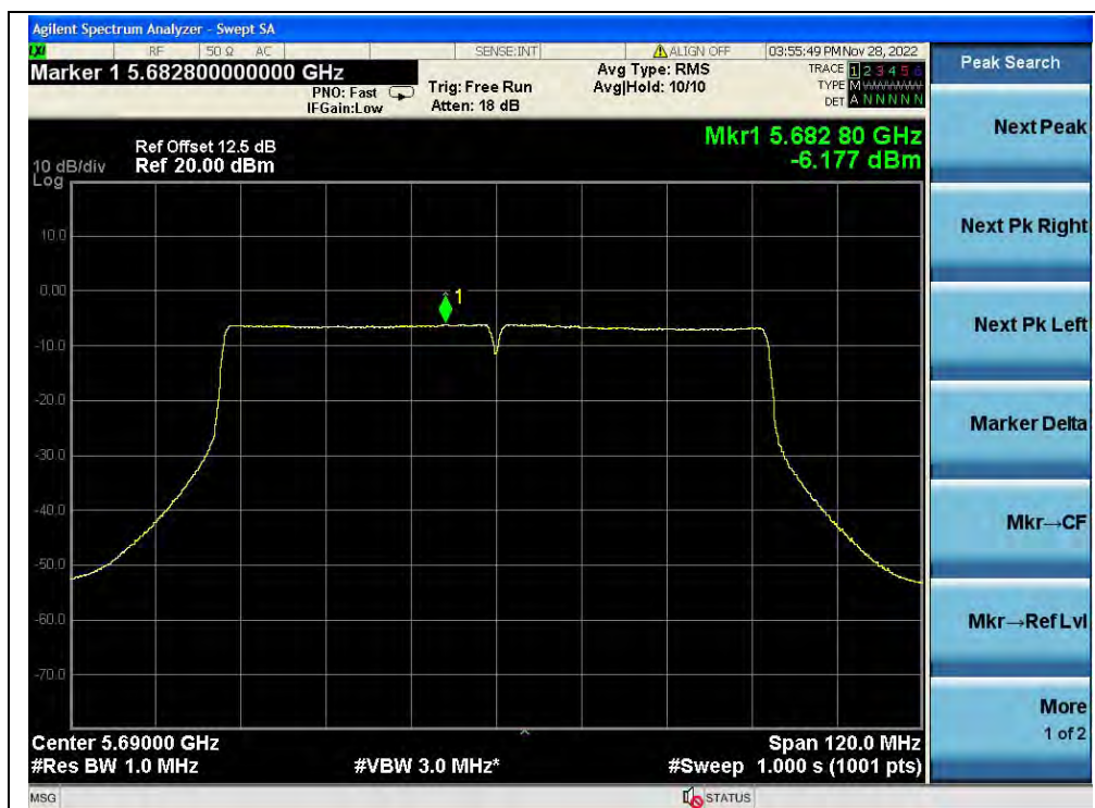
(Channel 138, 5690MHz, 802.11ac (VHT80), ANT0)
