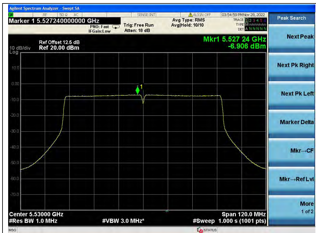
(Channel 106, 5530MHz, 802.11ac (VHT80), ANT0)
