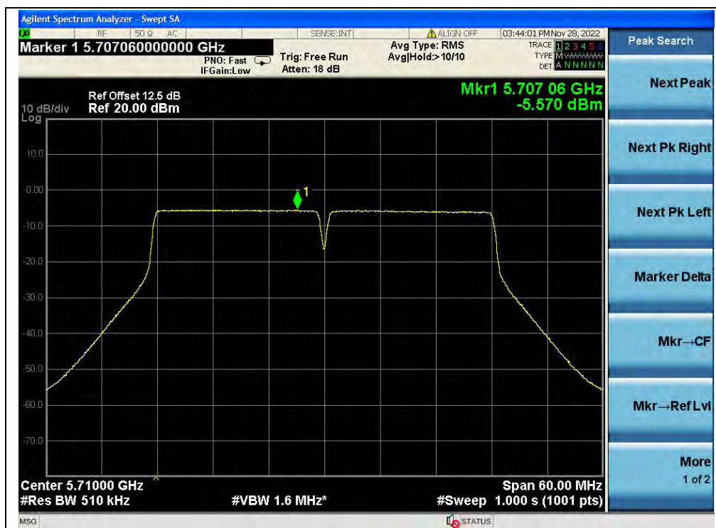
(Channel 142, 5710MHz, 802.11ac (VHT40), ANT0)
