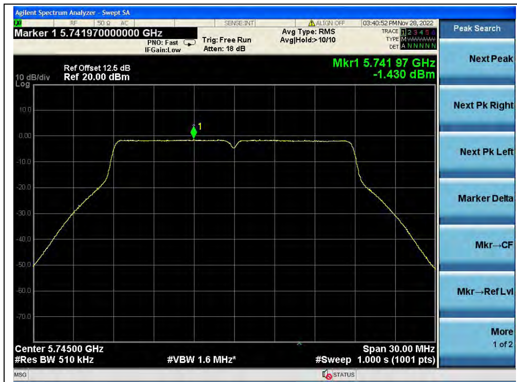
(Channel 149, 5745MHz, 802.11ac (VHT20), ANT0)
