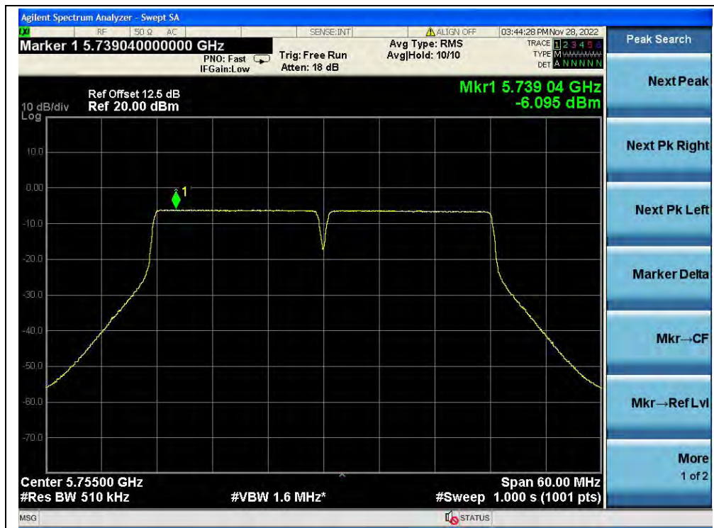
(Channel 151, 5755MHz, 802.11ac (VHT40), ANT0)
