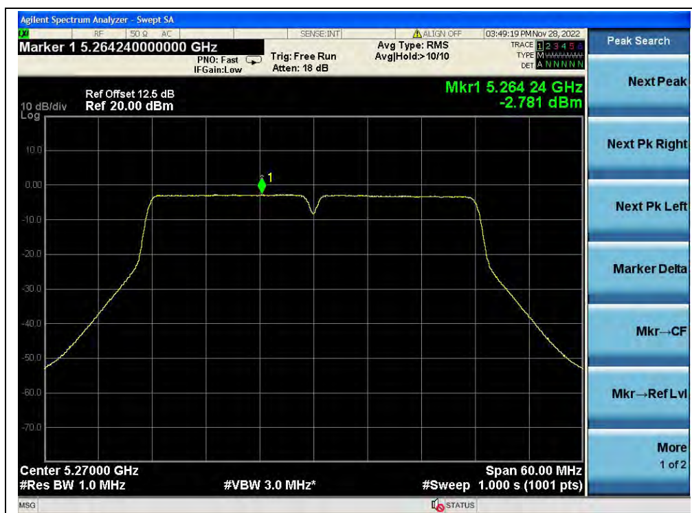
(Channel 54, 5270MHz, 802.11ac (VHT40), ANT0)
