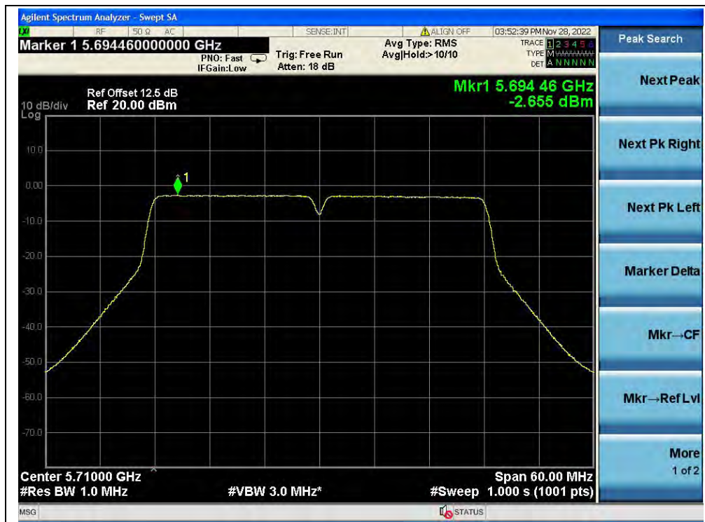
(Channel 142, 5710MHz, 802.11ac (VHT40), ANT0)
