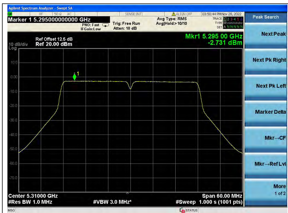
(Channel 62, 5310MHz, 802.11ac (VHT40), ANT0)
