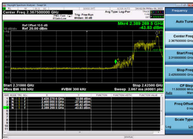
,Plot 2,Band Edge-802.11ax(HE20 _RU26_9),2412MHz,Ant7
