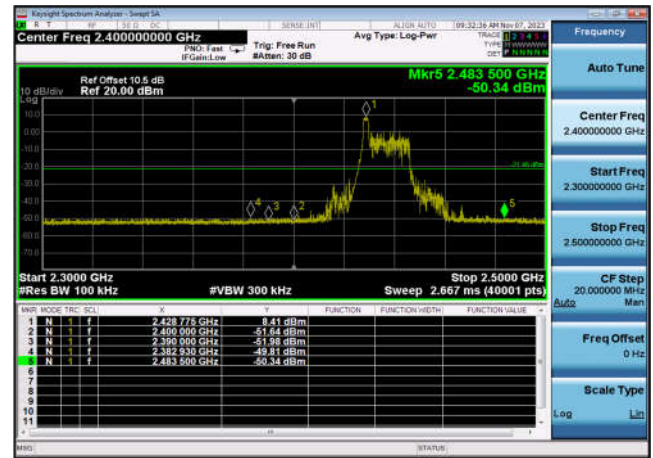
,Plot 2,Band Edge-802.11ax(HE20 _RU26_1),2462MHz,Ant6
