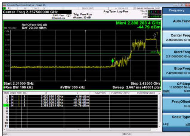
,Plot 2,Band Edge-802.11ax(HE20 _RU106_2),2412MHz,Ant7
