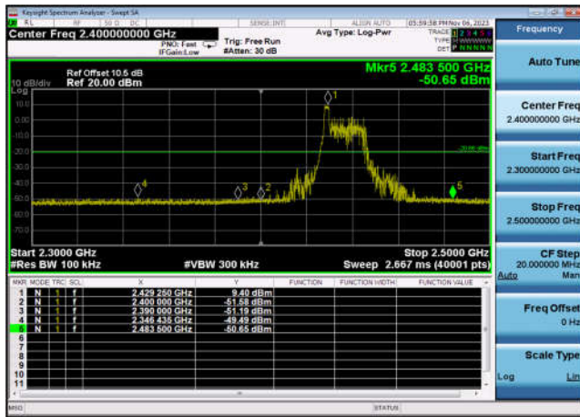
,Plot 2,Band Edge-802.11ax(HE20 _RU26_1),2462MHz,Ant7
