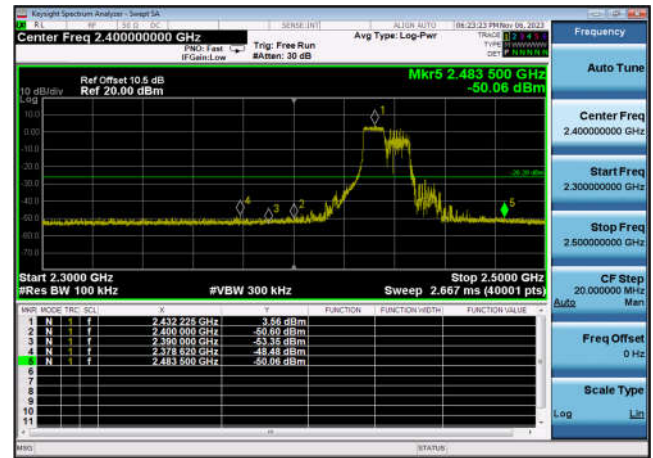
,Plot 2,Band Edge-802.11ax(HE20 _RU106_1),2462MHz,Ant7
