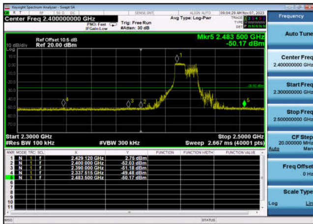
,Plot 2,Band Edge-802.11ax(HE20 _RU106_2),2412MHz,Ant7
