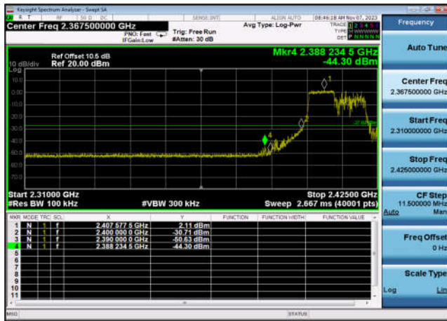
,Plot 2,Band Edge-802.11ax(HE20 _RU106_1),2437MHz,Ant6
