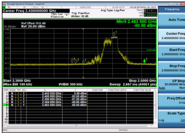
,Plot 2,Band Edge-802.11ax(HE20 _RU106_2),2462MHz,Ant7
