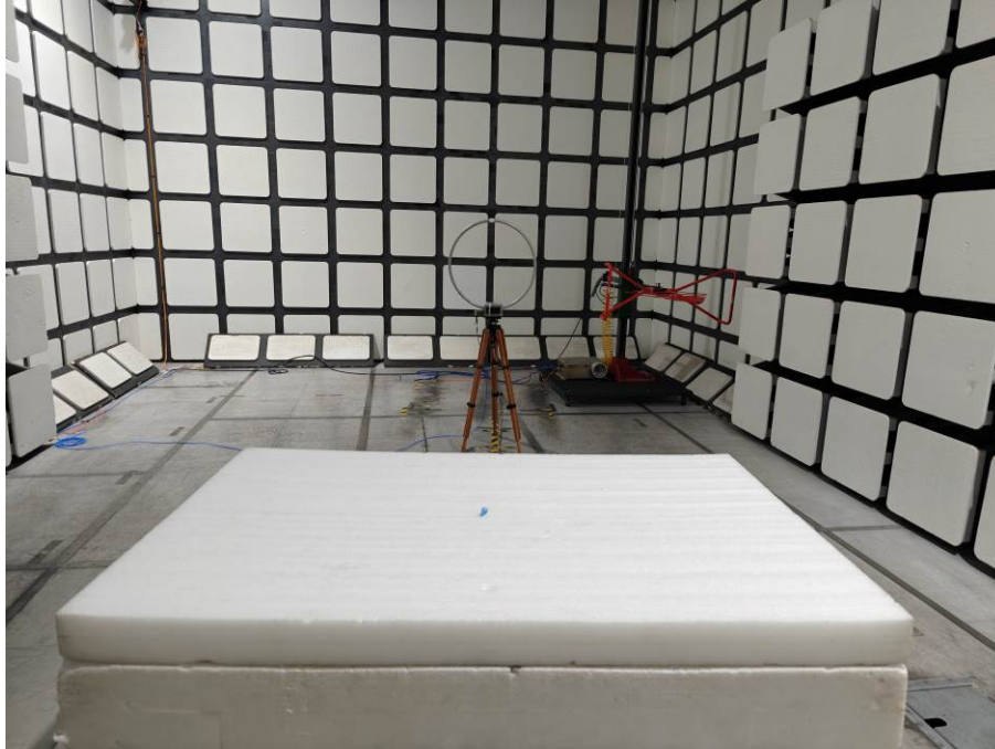
Radiated Emissions View (Below 30MHz)
