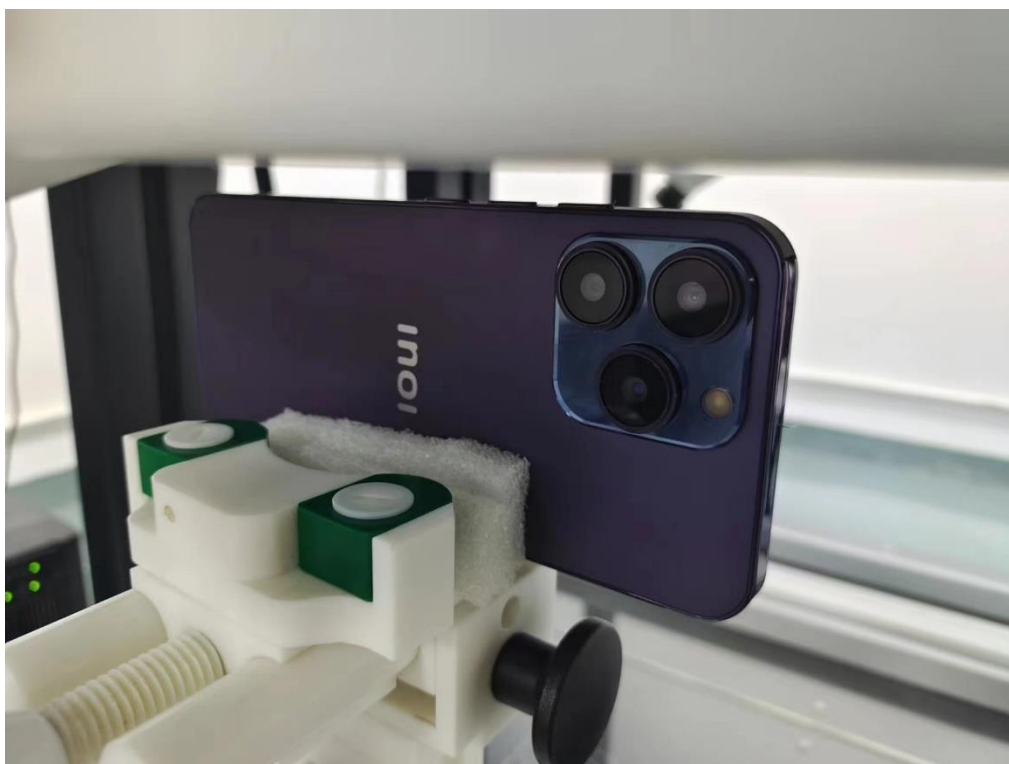
Body Right side (separation distance is 10mm)
