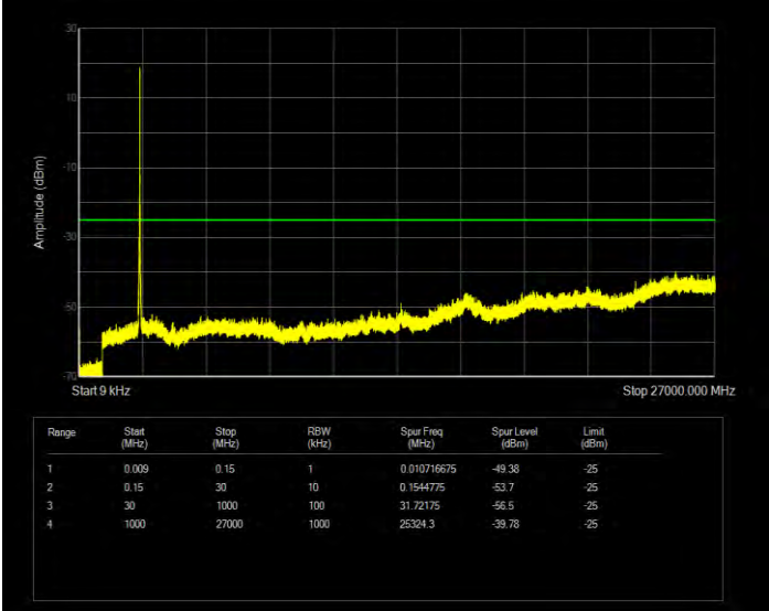
Band41 16QAM BW=10MHz Channel=41540 RB Size=50 Position=#0
