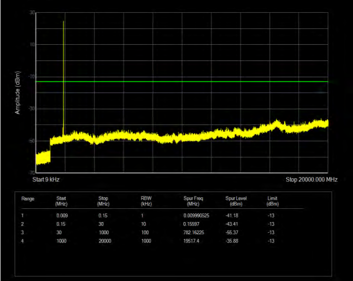
Band2 QPSK BW=10MHz Channel=18650 RB Size=50 Position=#0
