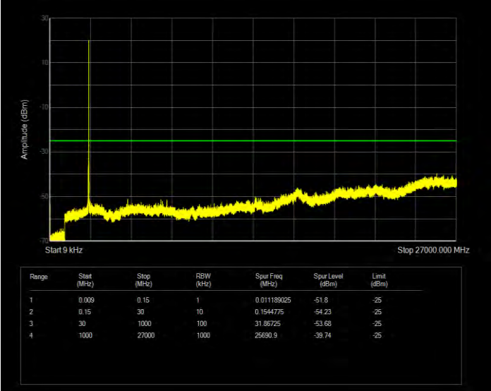
Band41 16QAM BW=5MHz Channel=41565 RB Size=25 Position=#0
