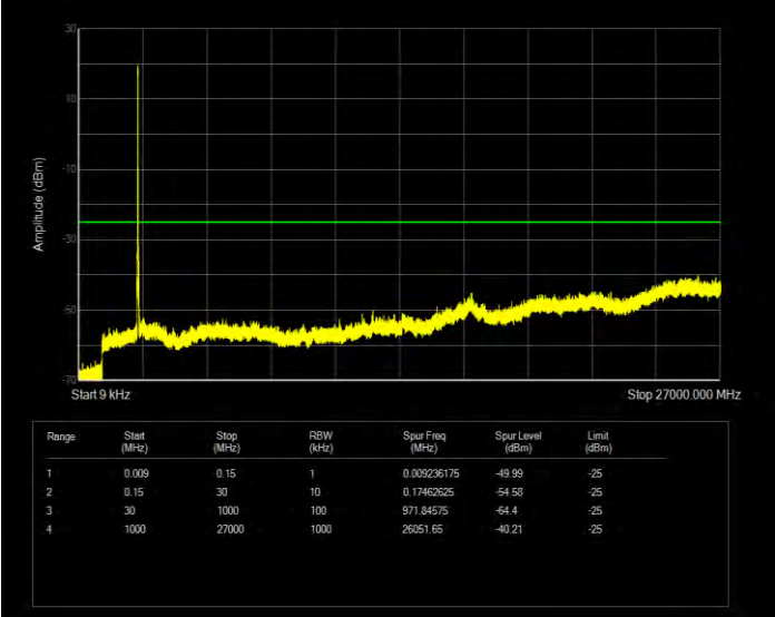
Band41 QPSK BW=10MHz Channel=39700 RB Size=50 Position=#0
