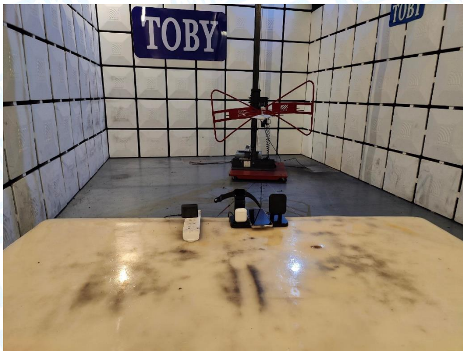
Photo of Setup for Radiated Emission (30M~1G)
