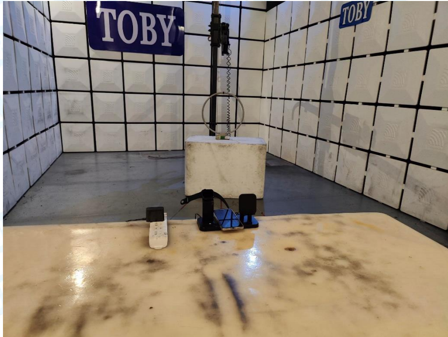
Photo of Setup for Radiated Emission (30M~1G)
