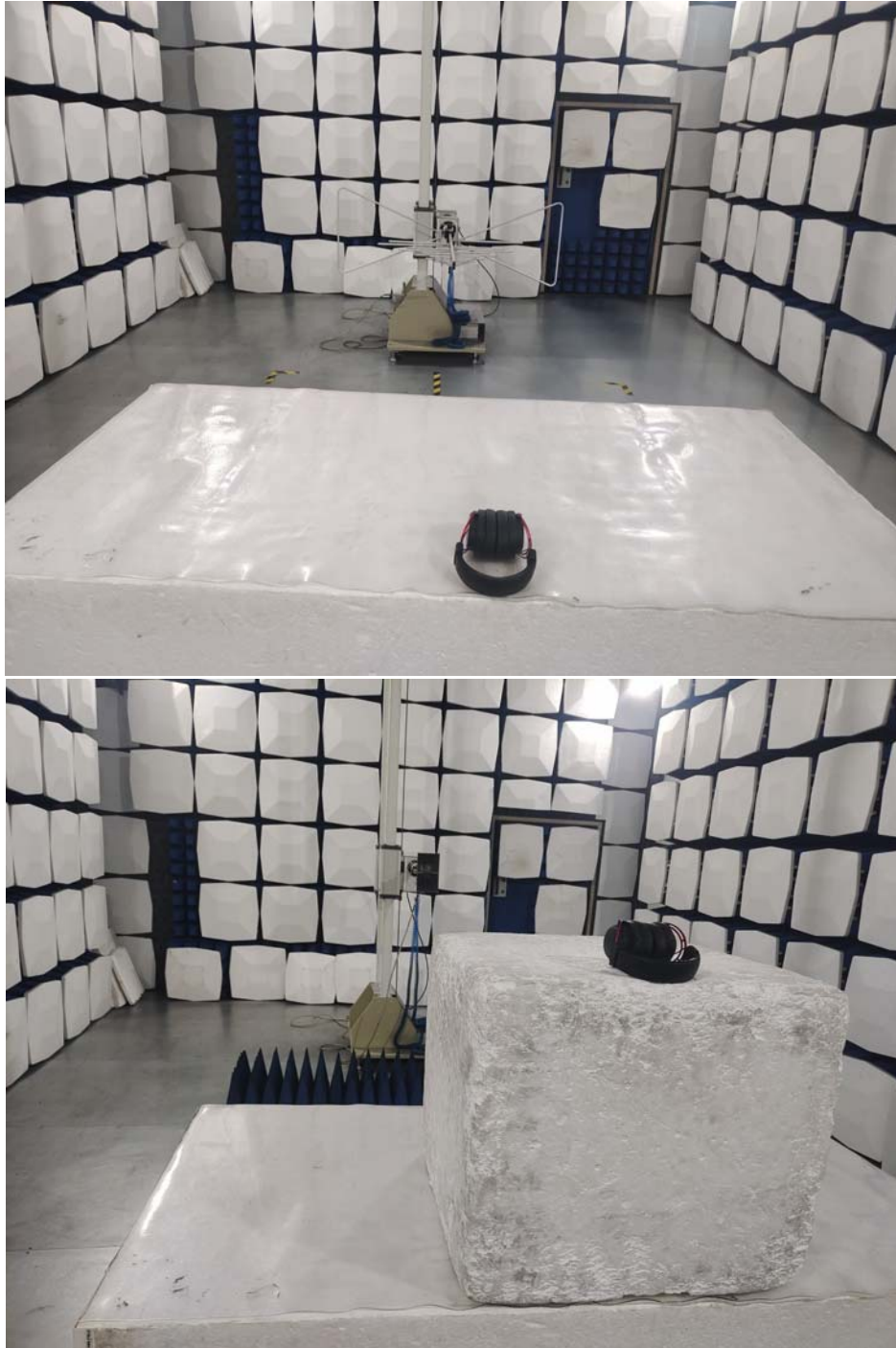
Radiated emission test view
