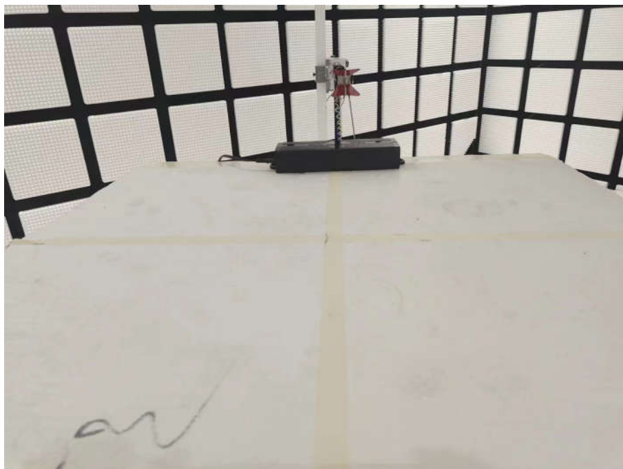
Radiated spurious emission Test Setup-2(Above 1GHz)
