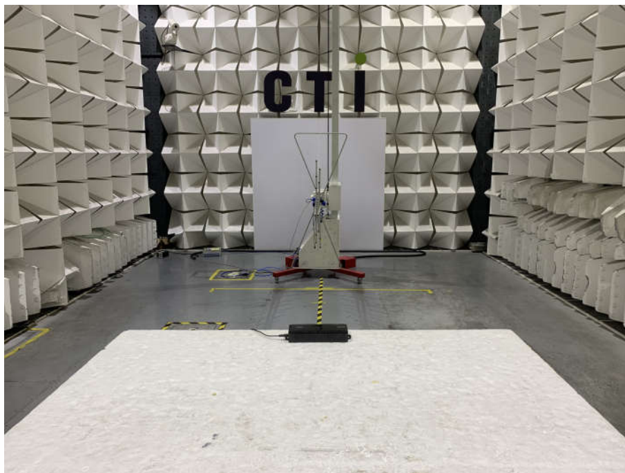
Radiated spurious emission Test Setup-1(Below 1GHz)
