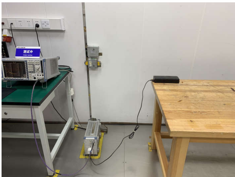
Conducted Emissions Test Setup
