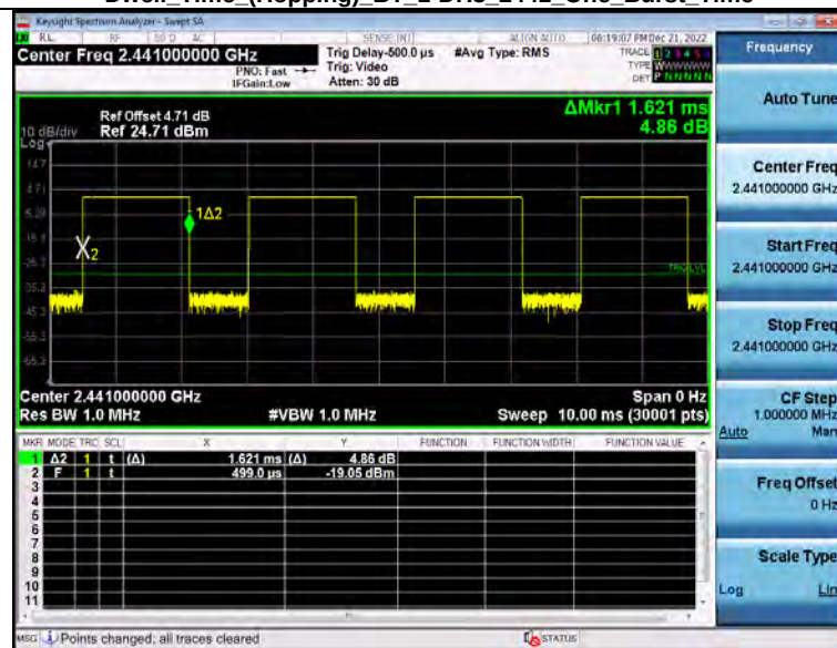
Dwell Time (Hopping) BT_1-DH3_2441_One Burst Time
