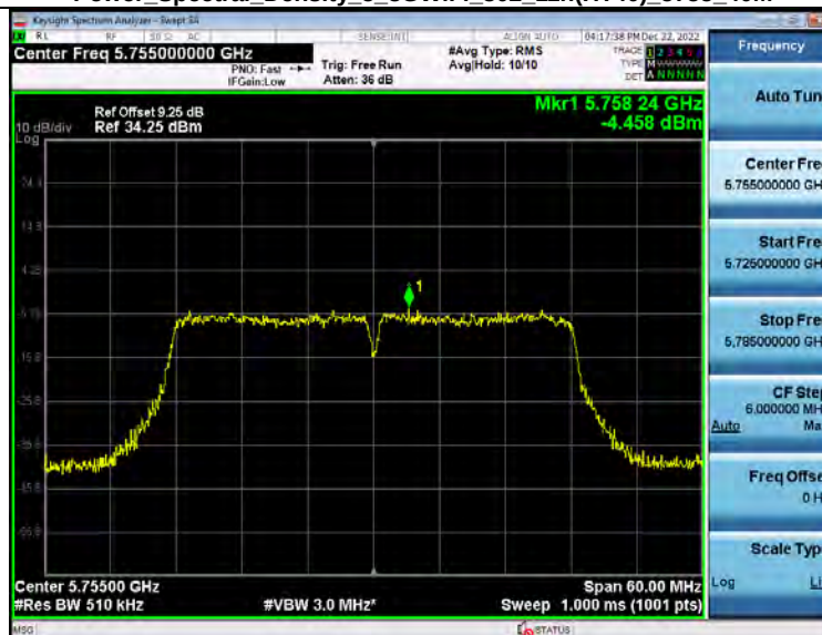
Power_Spectral_Density 5_8WiFi 802_11n(HT40)_5755_40M
