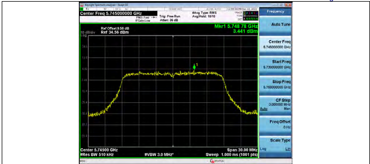
Power_Spectral_Density 5_8WiFi 802_11ac(VHT20)_5785_20M
