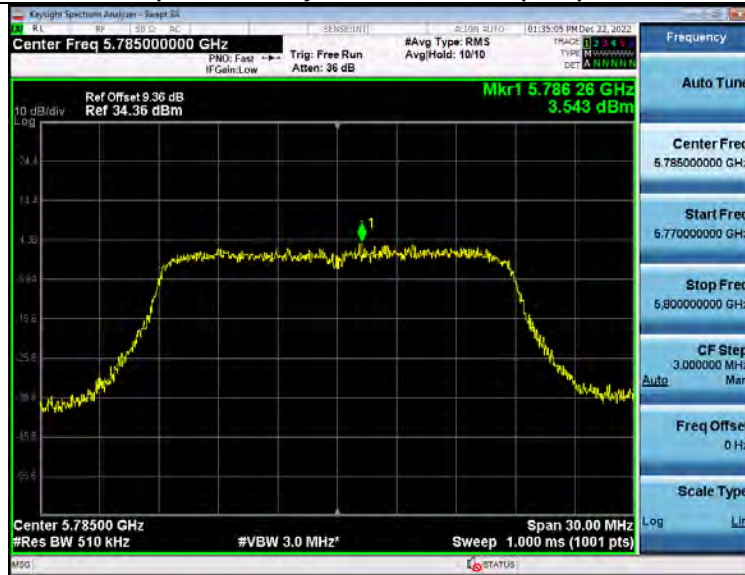
Power Spectral Density 5_8WiFi 802_11n(HT20) 5785_20M
