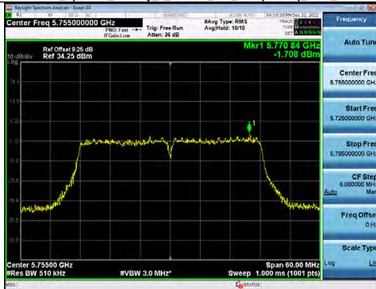
Power_Spectral_Density 5_8WiFi 802_11ac(VHT40) 5755_40M
