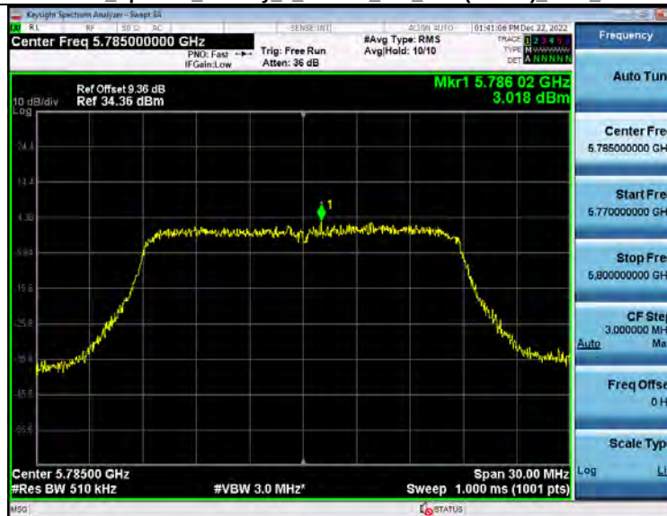
Power_Spectral_Density 5_8WiFi 802_11ac(VHT20)_5785_20M
