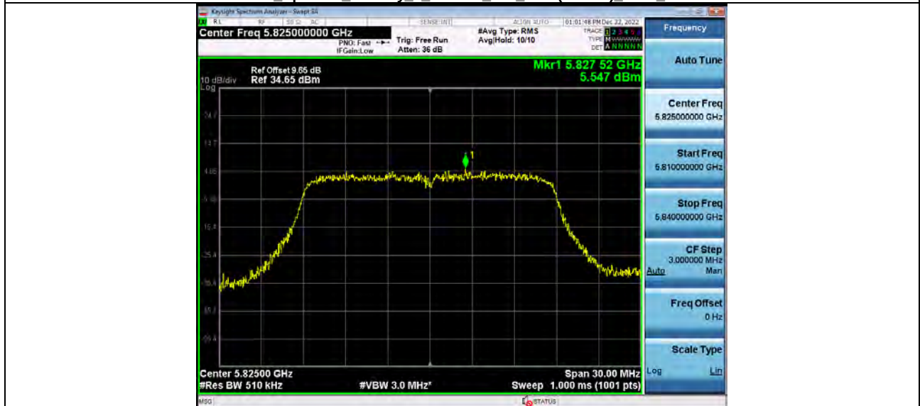
Power_Spectral_Density 5_8WiFi 802_11ac(VHT20)_5825_20M
