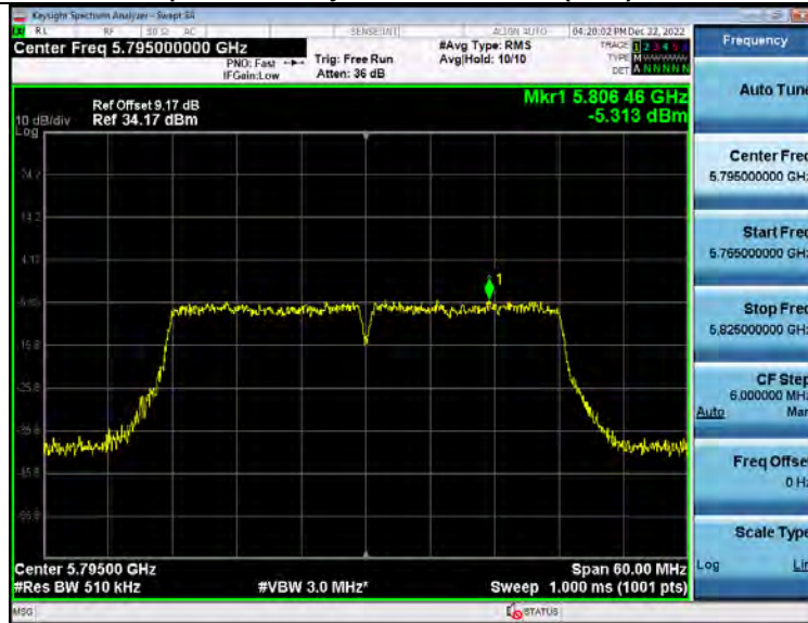
Power_Spectral_Density 5_8WiFi 802_11n(HT40) 5795_40M
