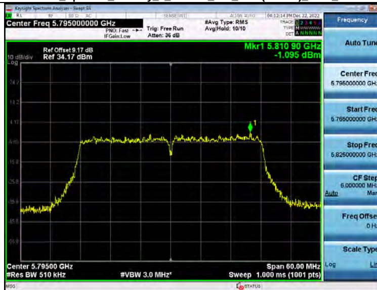
Power_Spectral_Density 5_8WiFi 802_11ac(VHT40) 5795_40M
