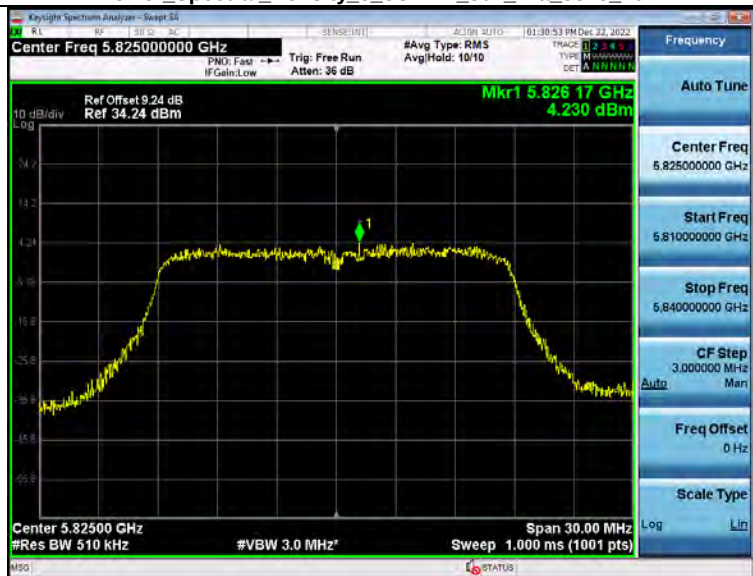
Power Spectral Density 5_8WiFi 802_11a 5825_20M
