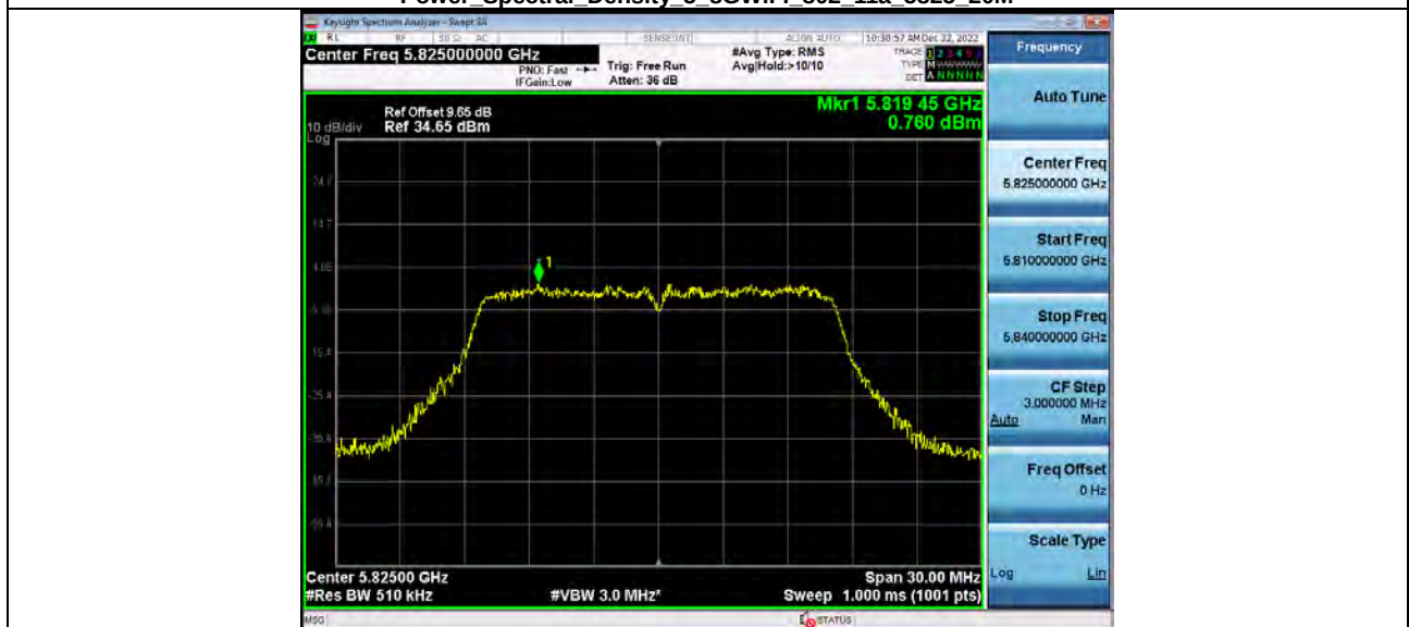
Power Spectral Density 5_8WiFi 802_11a 5825_20M
