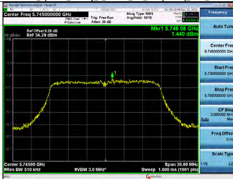
Power Spectral Density 5_8WiFi 802_11ac(VHT20) 5745_20M
