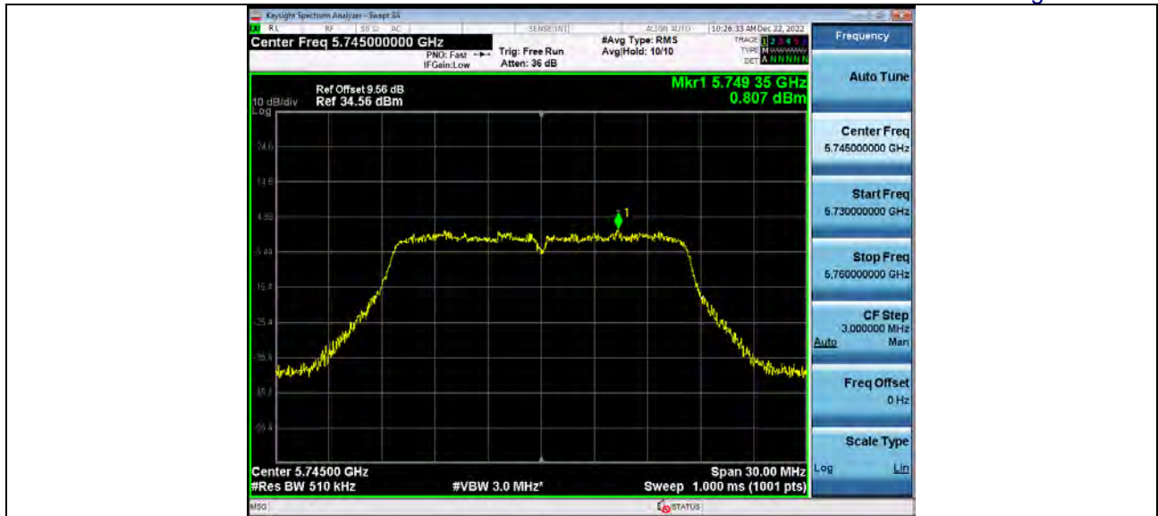
Power Spectral Density 5_8WiFi 802_11a 5785_20M
