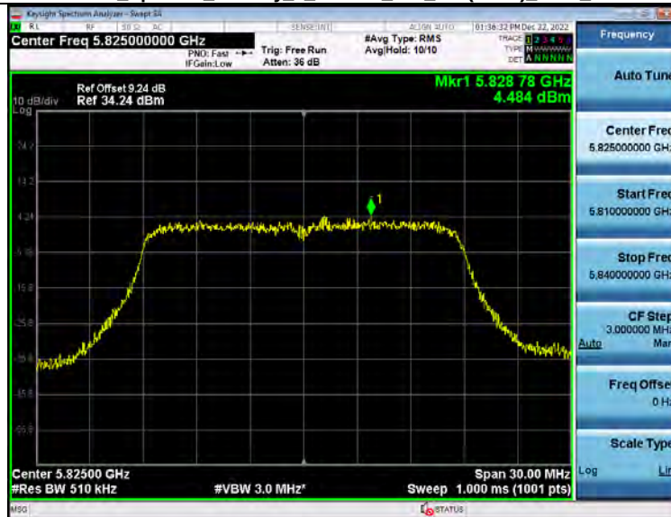
Power Spectral Density 5_8WiFi 802_11n(HT20) 5825_20M
