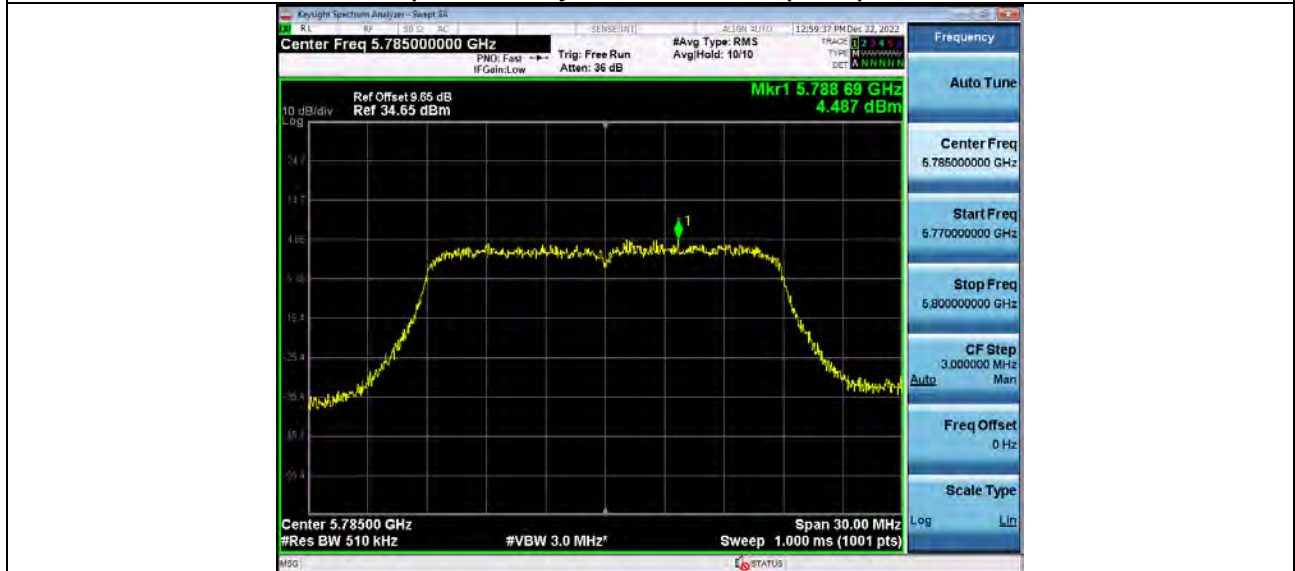
Power_Spectral_Density 5_8WiFi 802_11ac(VHT20)_5785_20M
