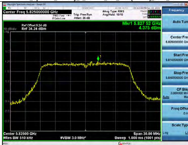
Power_Spectral_Density 5_8WiFi 802_11ac(VHT20)_5825_20M
