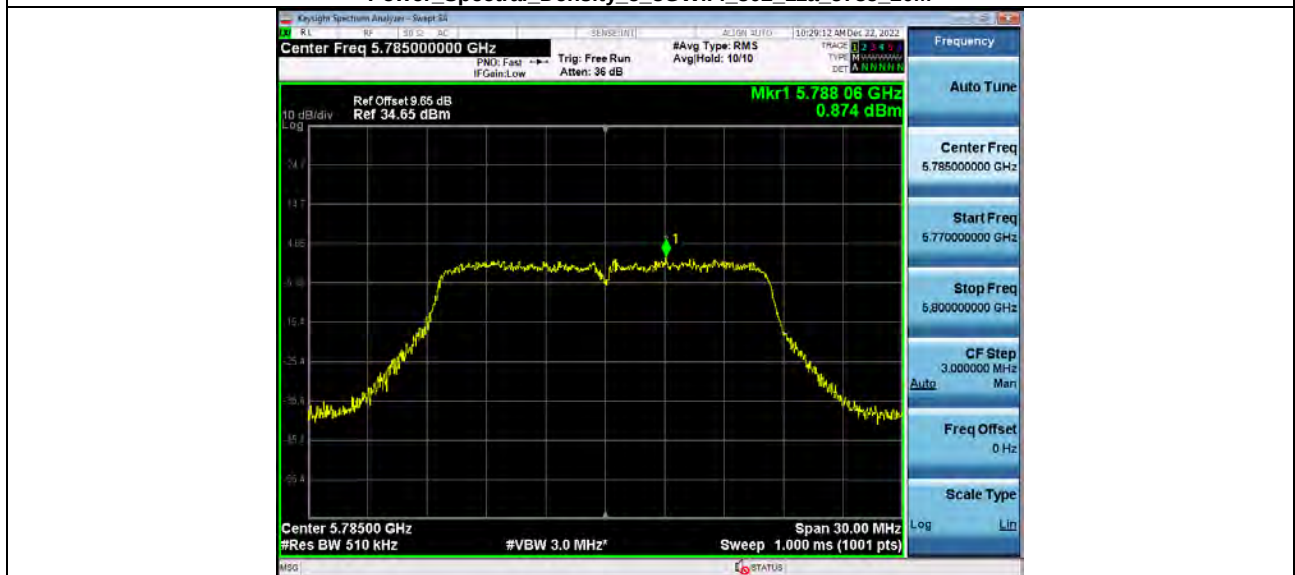
Power Spectral Density 5_8WiFi 802_11a 5785_20M
