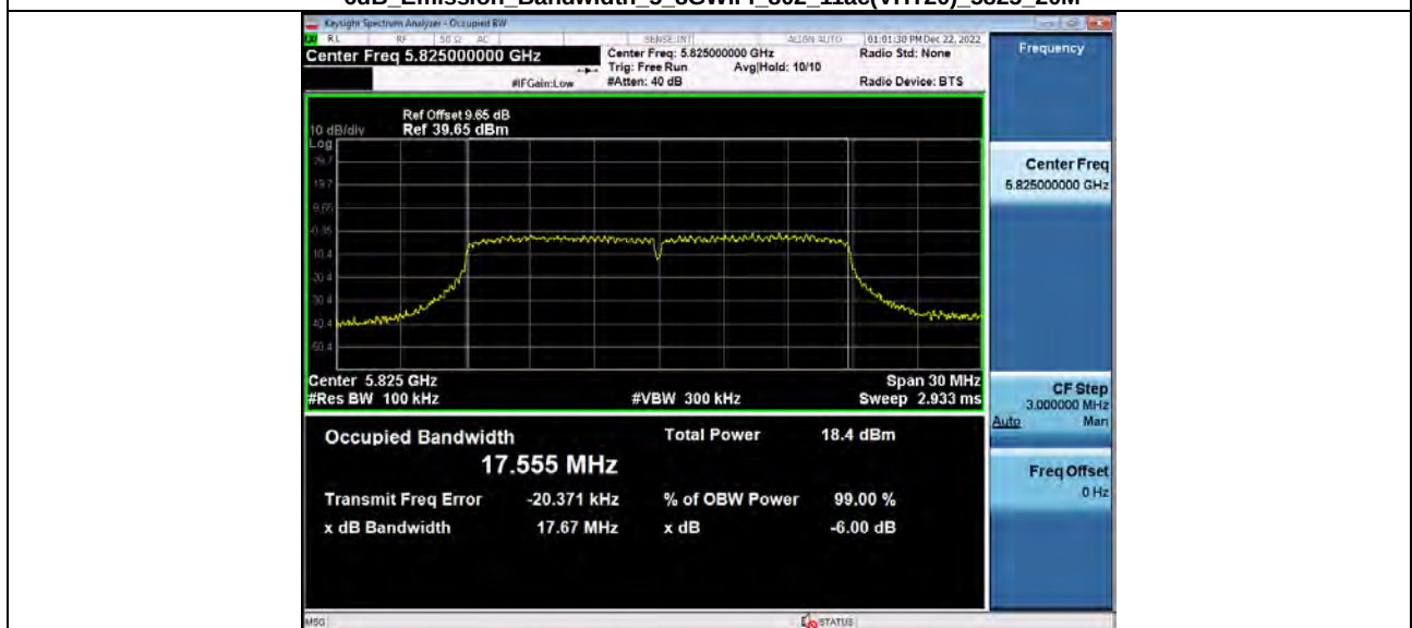
-6dB Emission Bandwidth 5_8WiFi 802_11ac(VHT20)_5825_20M
