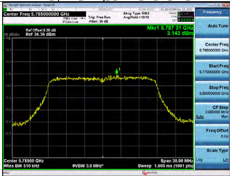
Power Spectral Density 5_8WiFi 802_11a 5785_20M
