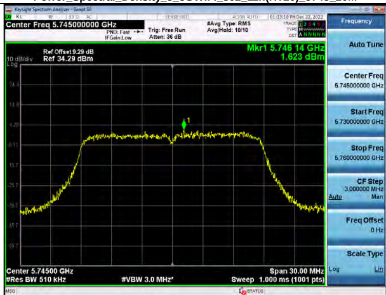
Power Spectral Density 5_8WiFi 802_11n(HT20) 5745_20M
