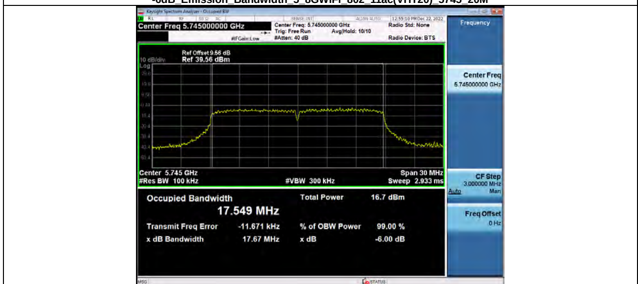
-6dB Emission Bandwidth 5_8WiFi 802_11ac(VHT20) 5785_20M
