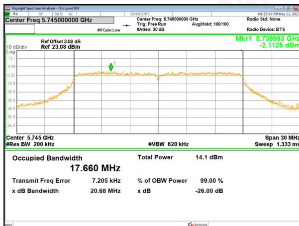
(802.11 n20) 99%Bandwidth plot on channel 149
