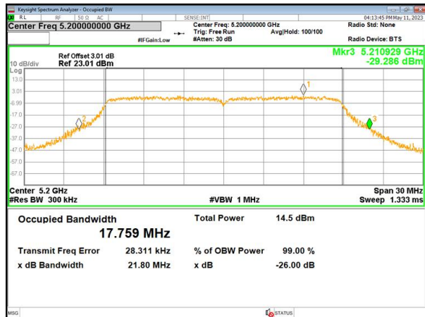
(802.11 n20) -26 dB Bandwidth plot on channel 48
