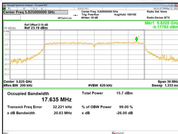
(802.11 n20) 99%Bandwidth plot on channel 165
