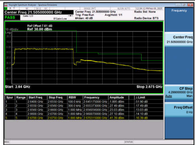
Band41_20MHz_QPSK_40340_100RB#0
