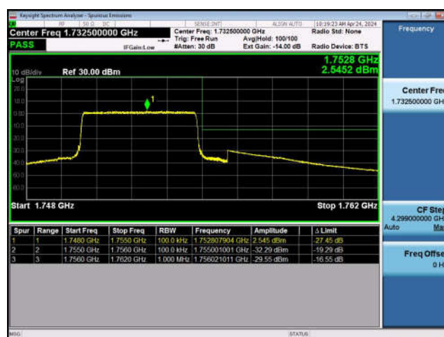
LTE Band 4-5MHz-QPSK-HCH-25RB#0
