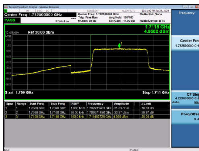
LTE Band 4-3MHz-QPSK-LCH-15RB#0
