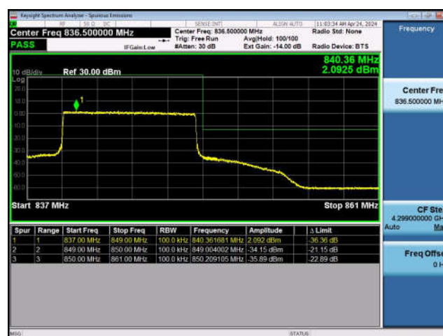
LTE Band 5-10MHz-QPSK-HCH-50RB#0
