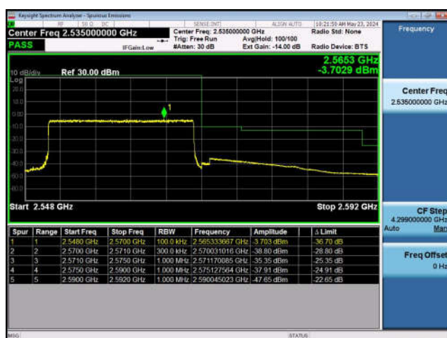
LTE Band 7-20MHz-QPSK-HCH-100RB#0
