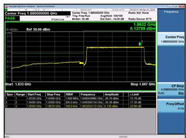
LTE Band 2-15MHz-QPSK-LCH-75RB#0
