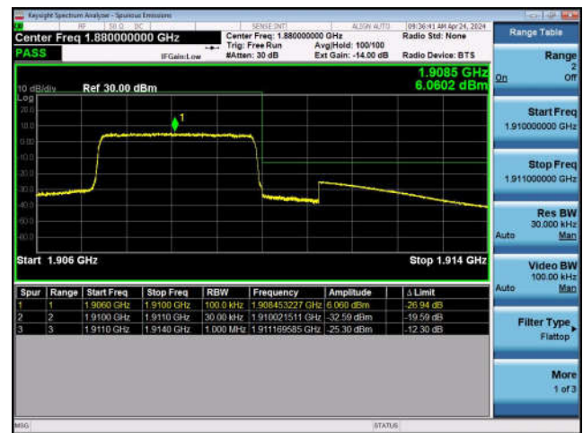
LTE Band 2-5MHz-QPSK-LCH-25RB#0
