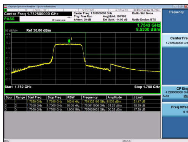
LTE Band 4-3MHz-QPSK-LCH-15RB#0
