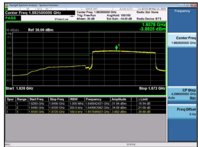
LTE Band 25-20MHz-QPSK-HCH-100RB#0
