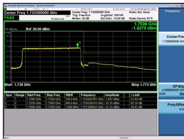
LTE Band 4-20MHz-QPSK-LCH-100RB#0
