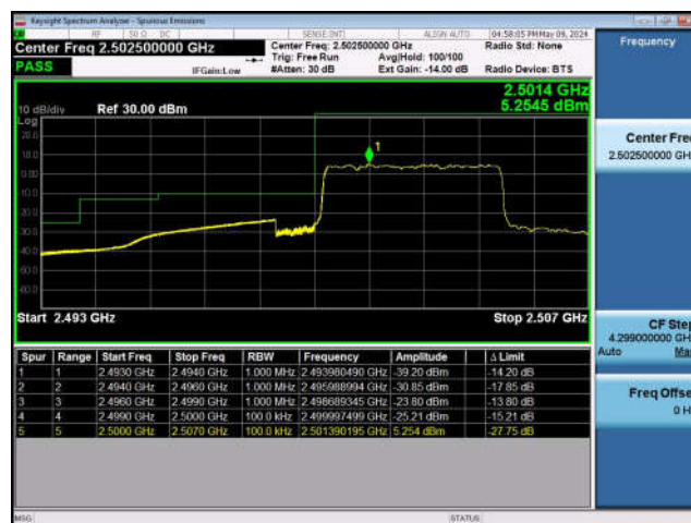
LTE Band 7-5MHz-QPSK-HCH-25RB#0
