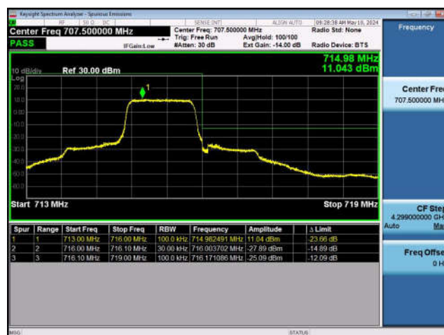
LTE Band 12-3MHz-QPSK-LCH-15RB#0
