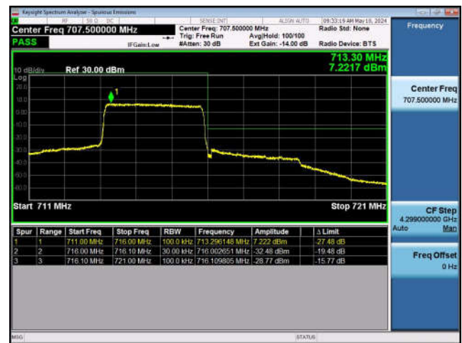
LTE Band 12-5MHz-QPSK-LCH-25RB#0
