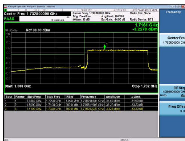
LTE Band 4-20MHz-QPSK-HCH-100RB#0
