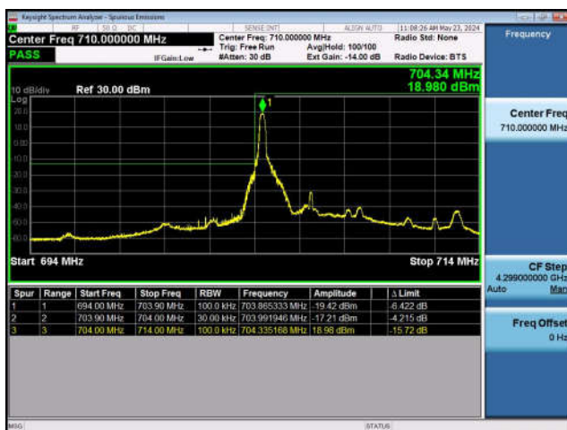
LTE Band 17-5MHz-QPSK-HCH-1RB#24
