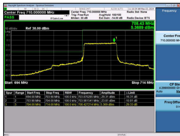
LTE Band 17-5MHz-QPSK-HCH-25RB#0
