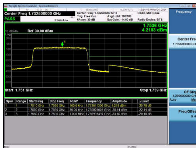
LTE Band 4-5MHz-QPSK-LCH-25RB#0
