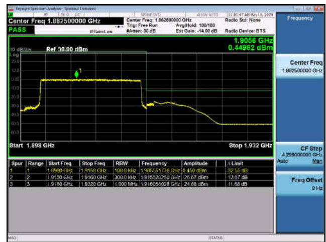
LTE Band 25-20MHz-QPSK-LCH-100RB#0
