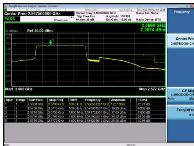
LTE Band 7-10MHz-QPSK-LCH-50RB#0
