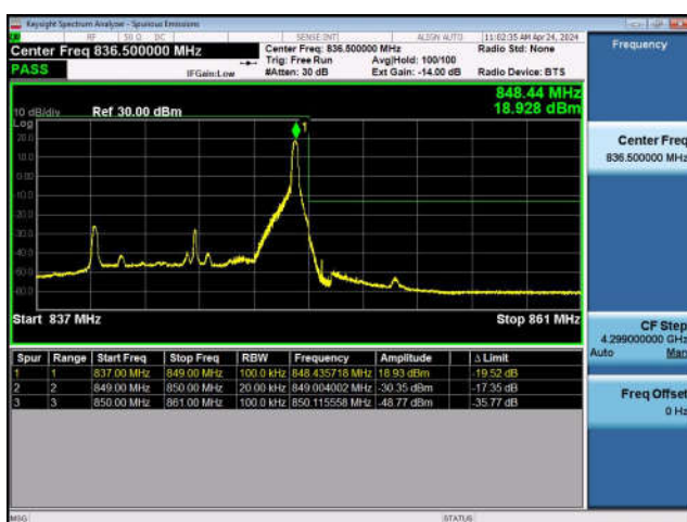
LTE Band 5-10MHz-QPSK-HCH-1RB#49
