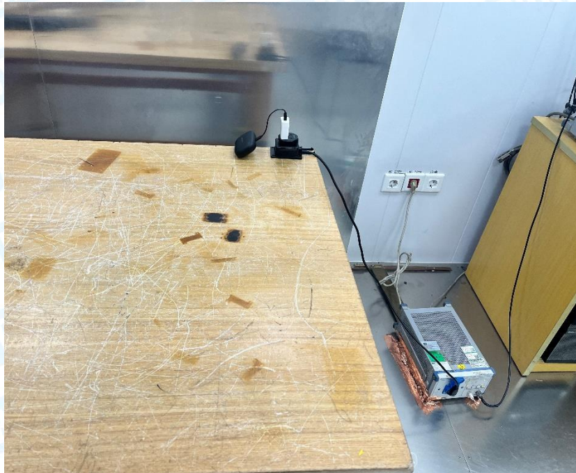
Photo of Setup for Radiated Emission (30MHz~1GHz)
