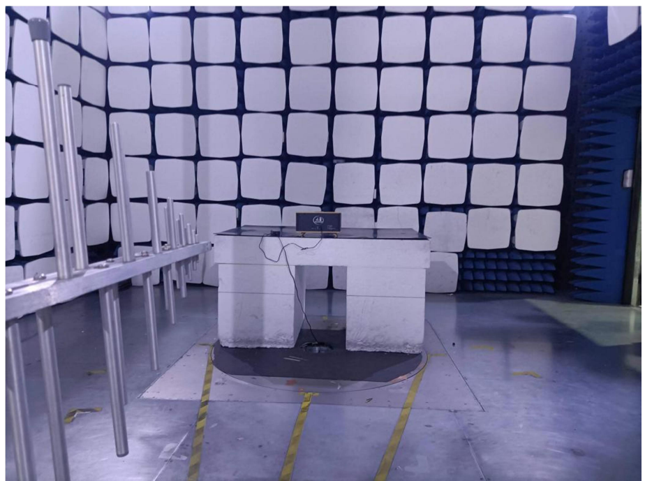
Radiation Emission Test Setup (30MHz to 1GHz)
