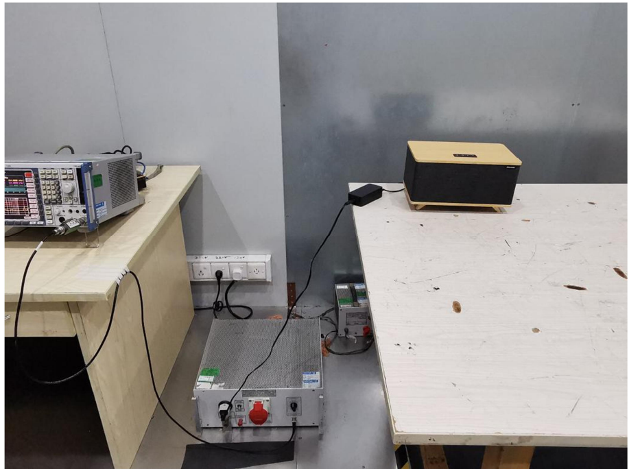
Conducted Emission Test Setup
