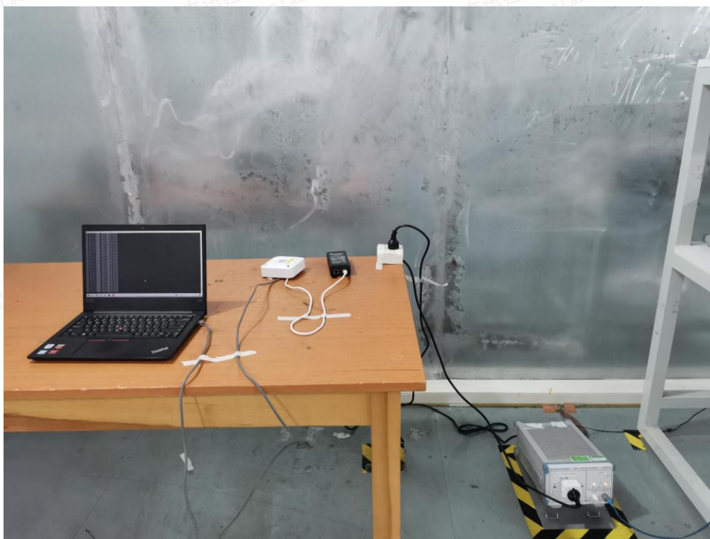
Photo of Power Line Conducted Measurement
