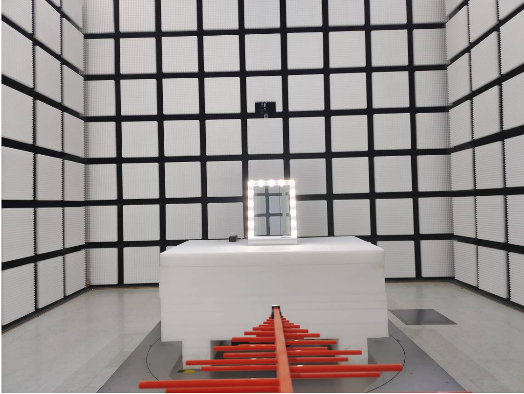
Radiated Emission Above 1GHz View
