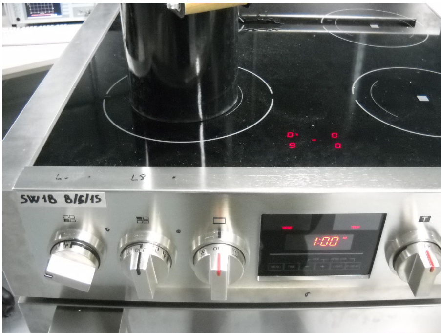
Figure 4: Disturbance Voltage measurement
