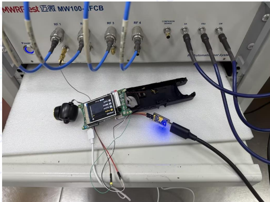
Photo of Setup for Conducted Measurements
