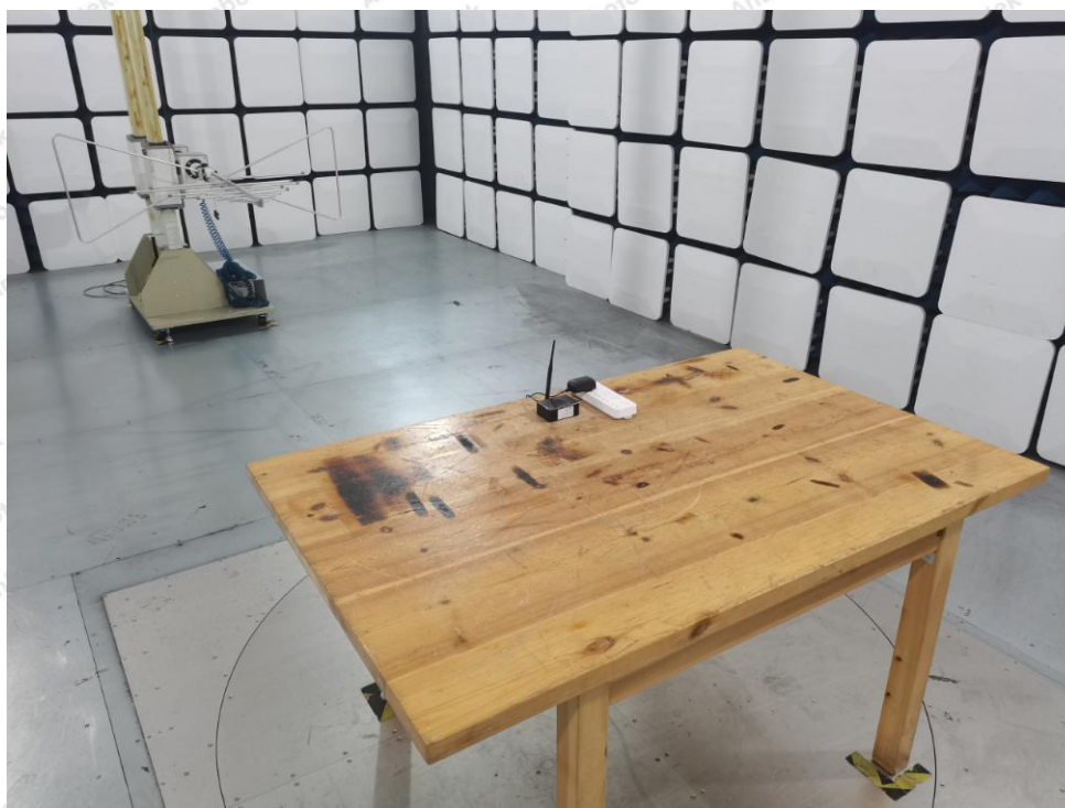
Photo of Radiation Emission Test
