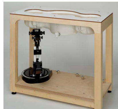
Picture C.10: SAM Twin Phantom
