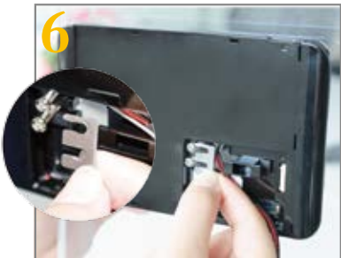
Insert reinforced shim ( as show in figure, thinner side is up)
