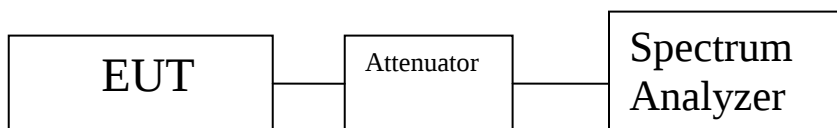
Figure 3. Peak Power Output Test Setup
