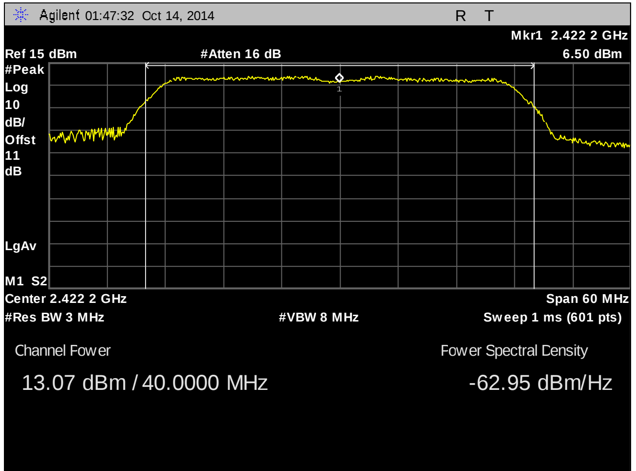
Plot 34. Peak Power Output, n Mode, 40 MHz, Low Channel
