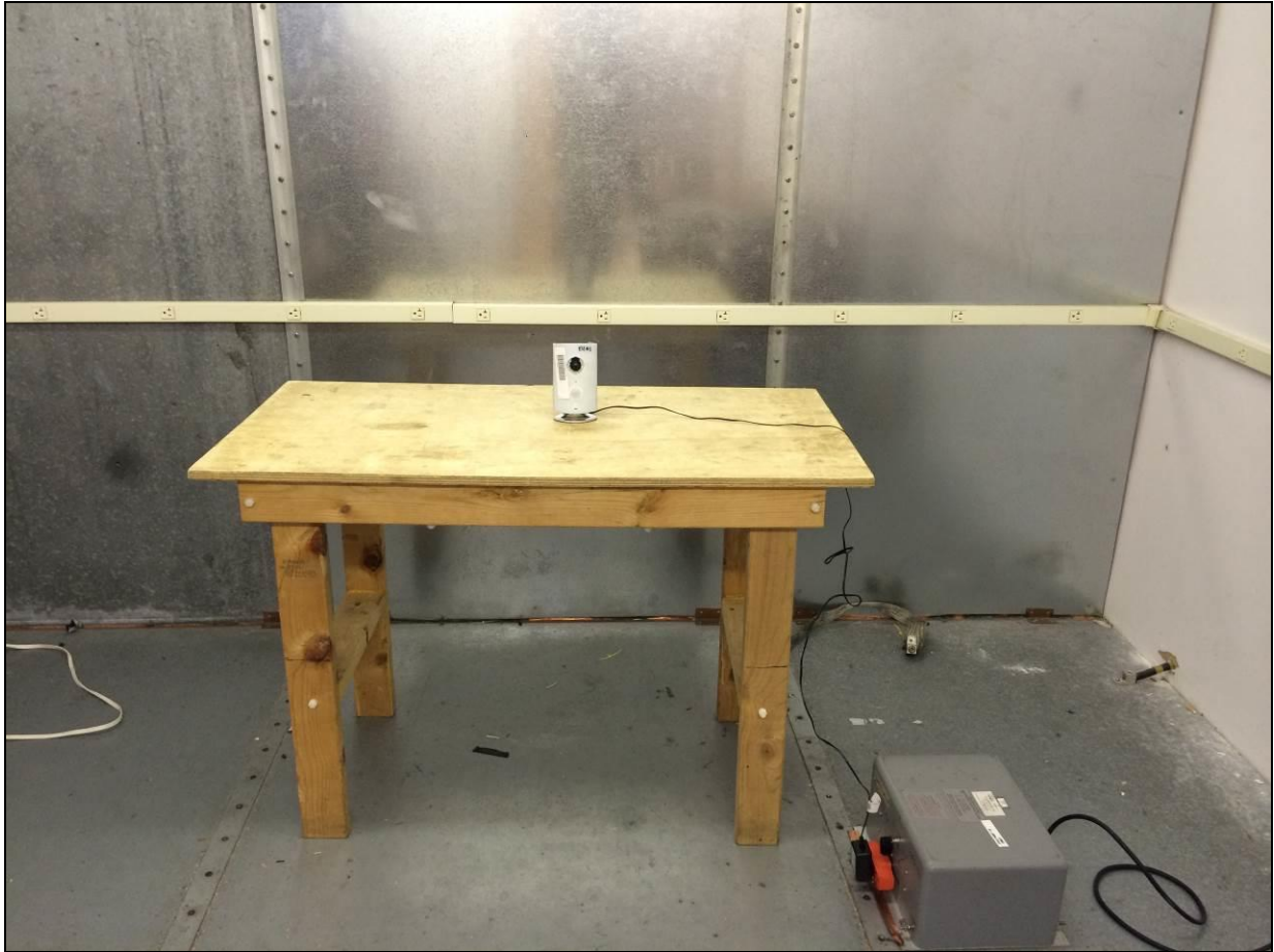
Photograph 1. Conducted Emissions, Test Setup
