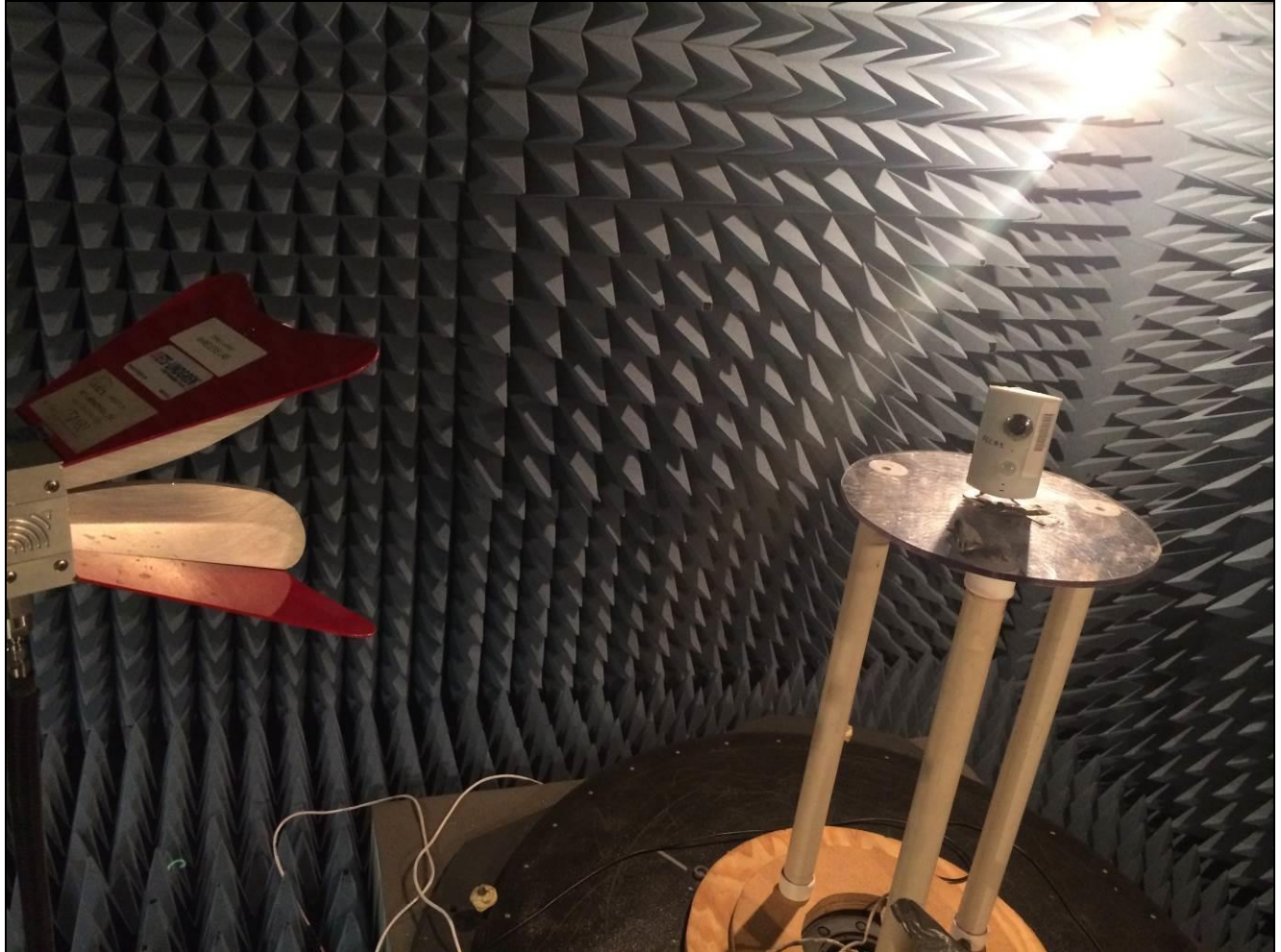
Photograph 4. Radiated Spurious Emissions, Test Setup, 1
