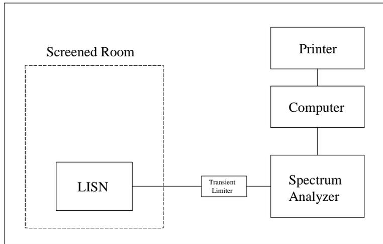
**A1.2 Direct Connection at the Antenna Port Tests**
