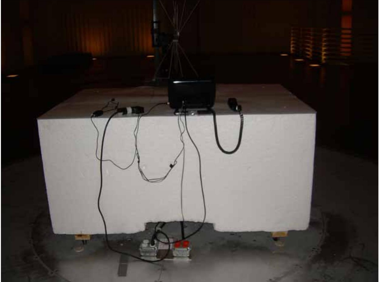
Photograph 3 – Front View Conducted Disturbance Worst Case Configuration
