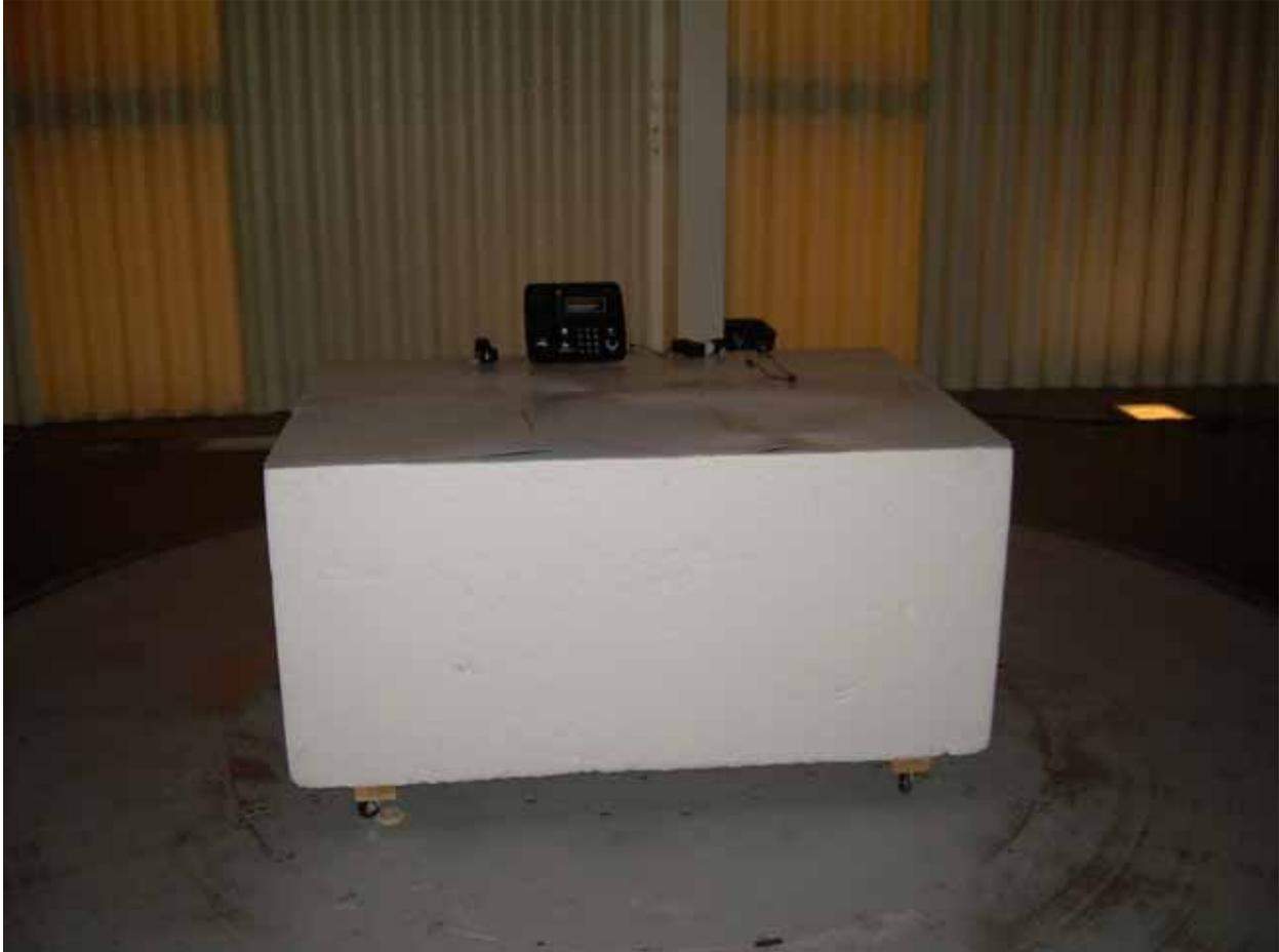
Photograph 2 – Back View Radiated Disturbance Worst Case Configuration
