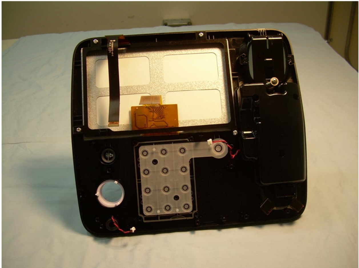
Internal View with PCBs Removed
