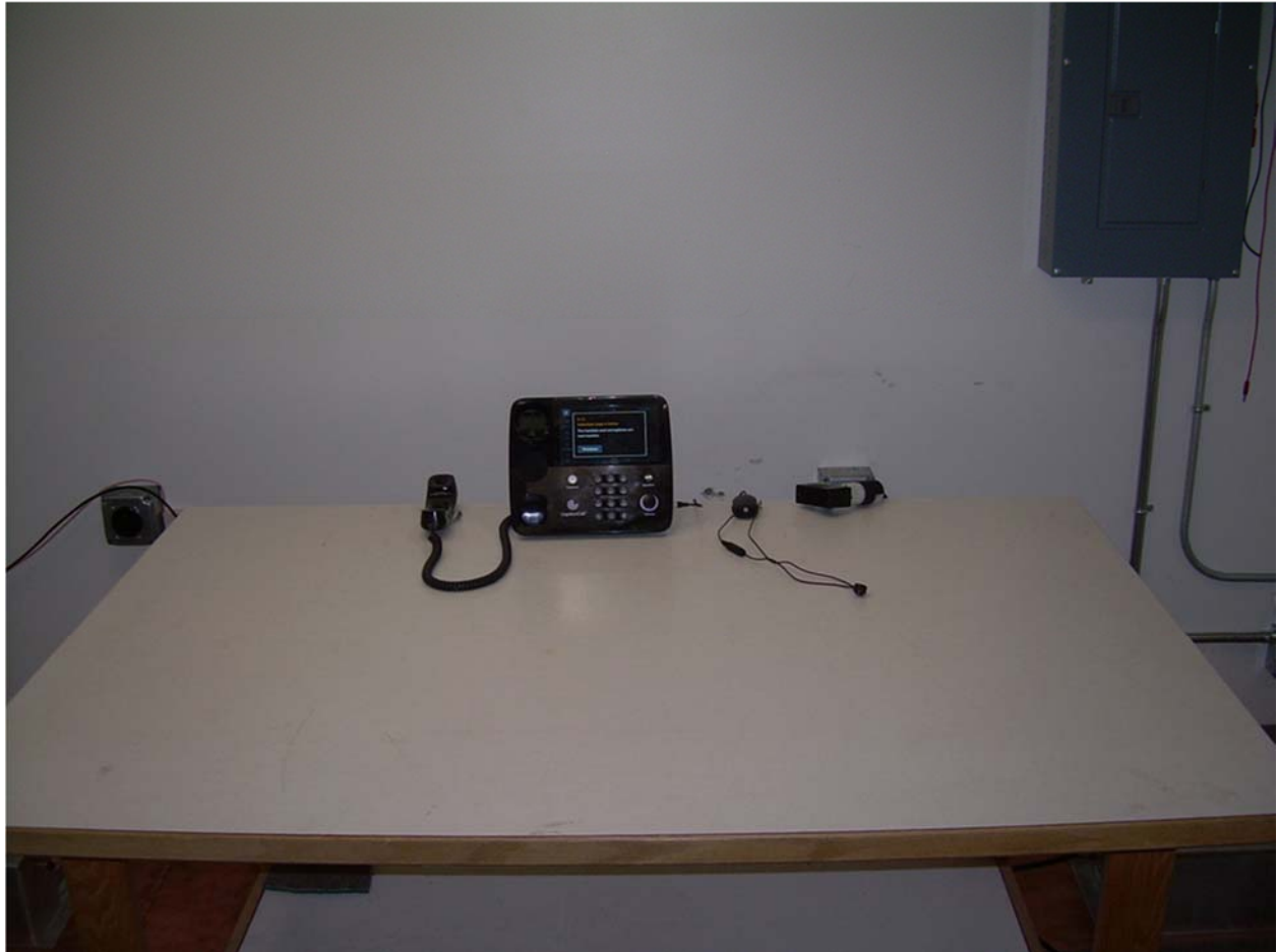
Front View Conducted Disturbance Worst Case Configuration
