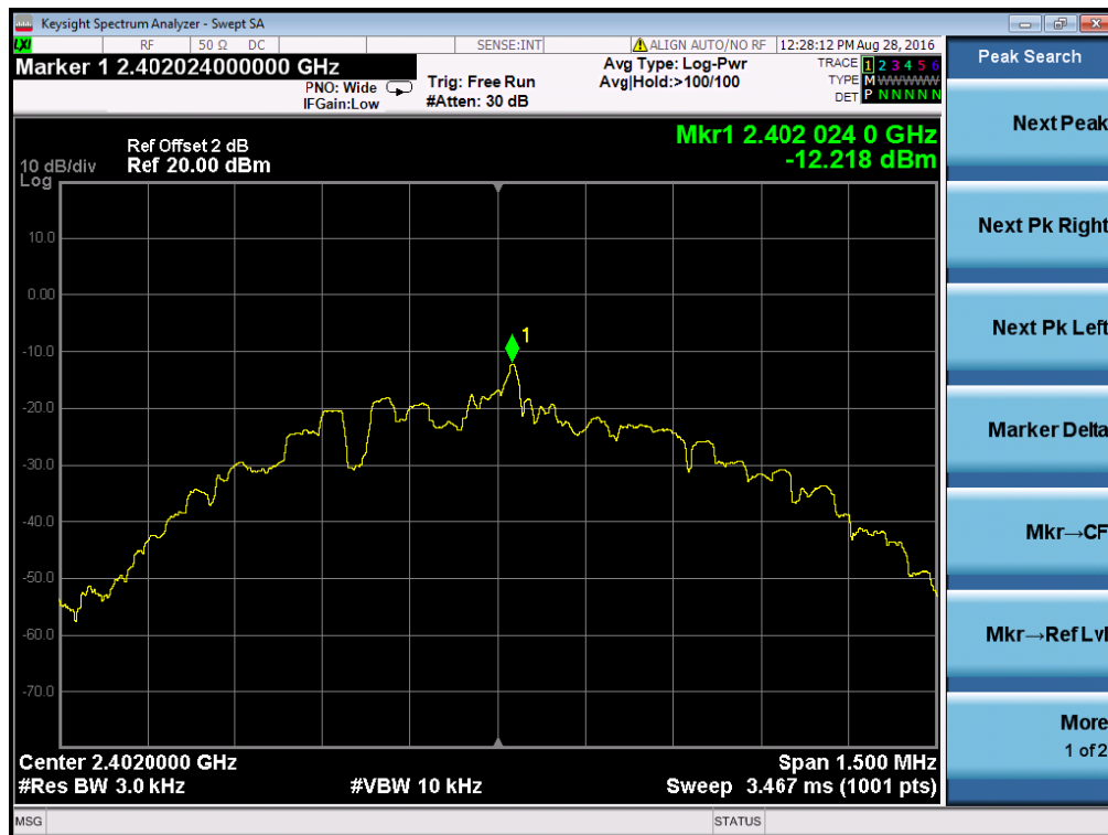
PSD Plot on Channel 0
