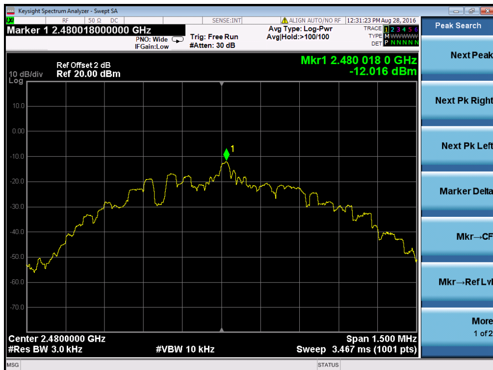
PSD Plot on Channel 39
