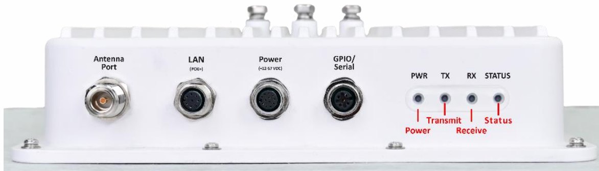
FIGURE 1 - Connector Faceplate Arrangement
