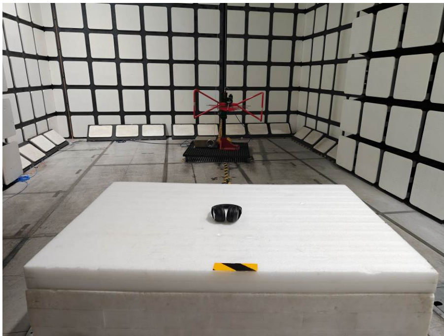
Radiated Emissions View (Below 1 GHz)
