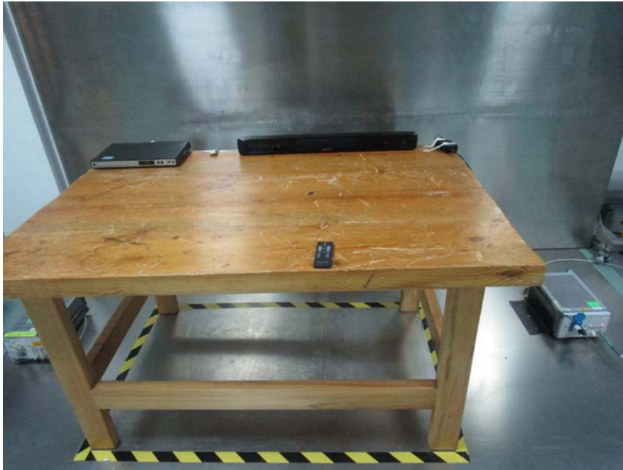
Conducted Emission--Front View
