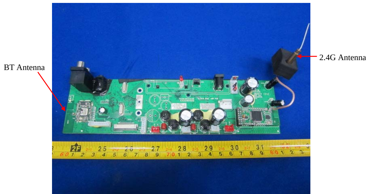
EUT –Main Board Top View
