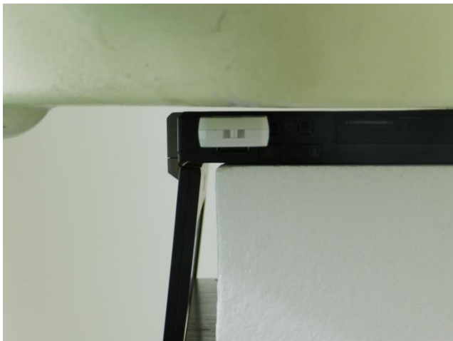
Horizontal Up, Test Separation 5 mm
