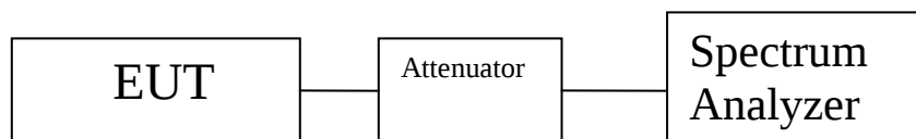
Figure 4. Block Diagram, Conducted Spurious Emissions Test Setup
