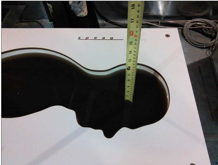
Figure 17: 5GHz head tissue simulating fluid
