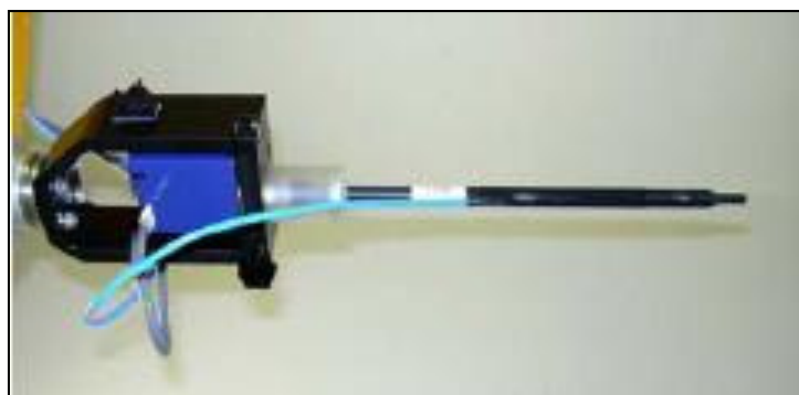
Figure 11: Electric field probe
