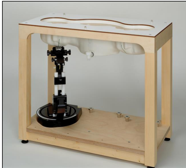
Figure 12: Specific anthropomorphic mannequin twin phantom
