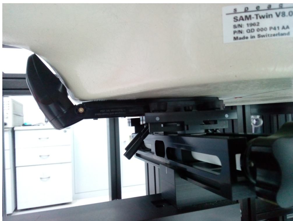
Front to Phantom (0mm)Setup Photo
