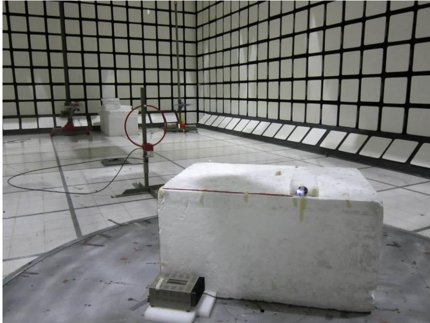
RADIATED PHOTO (BELOW 1 GHz) 3m – Wired
