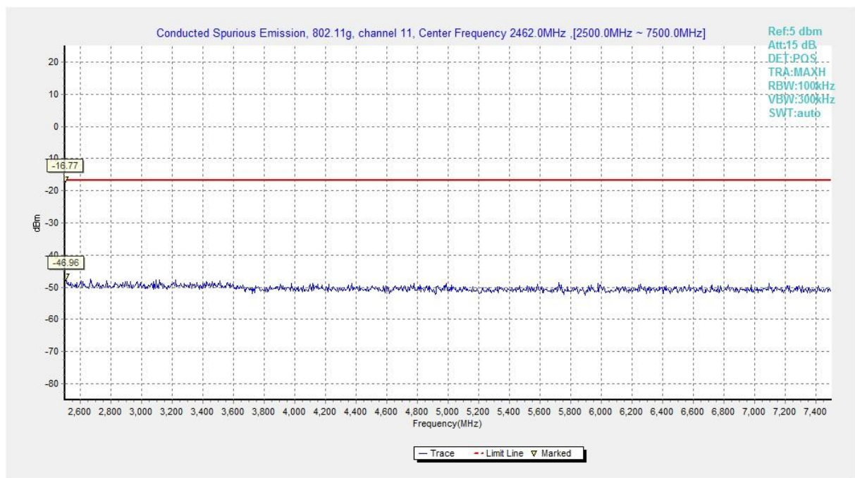
Fig.A.7.1.44 Conducted Spurious Emission (802.11g, Ch11, 2.5 GHz-7.5 GHz)
