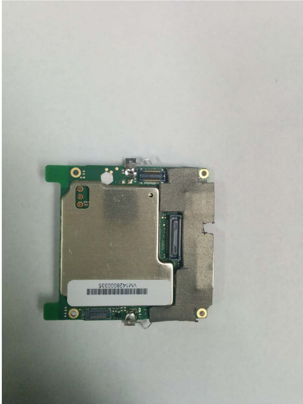
Figure 14: Main Board - Top View With Ferrite Sheet
