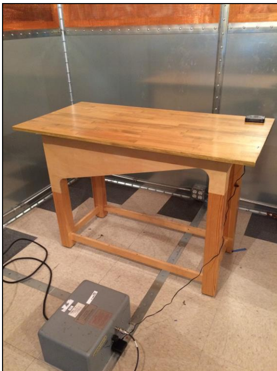
Photograph 1. Conducted Emissions, Test Setup
