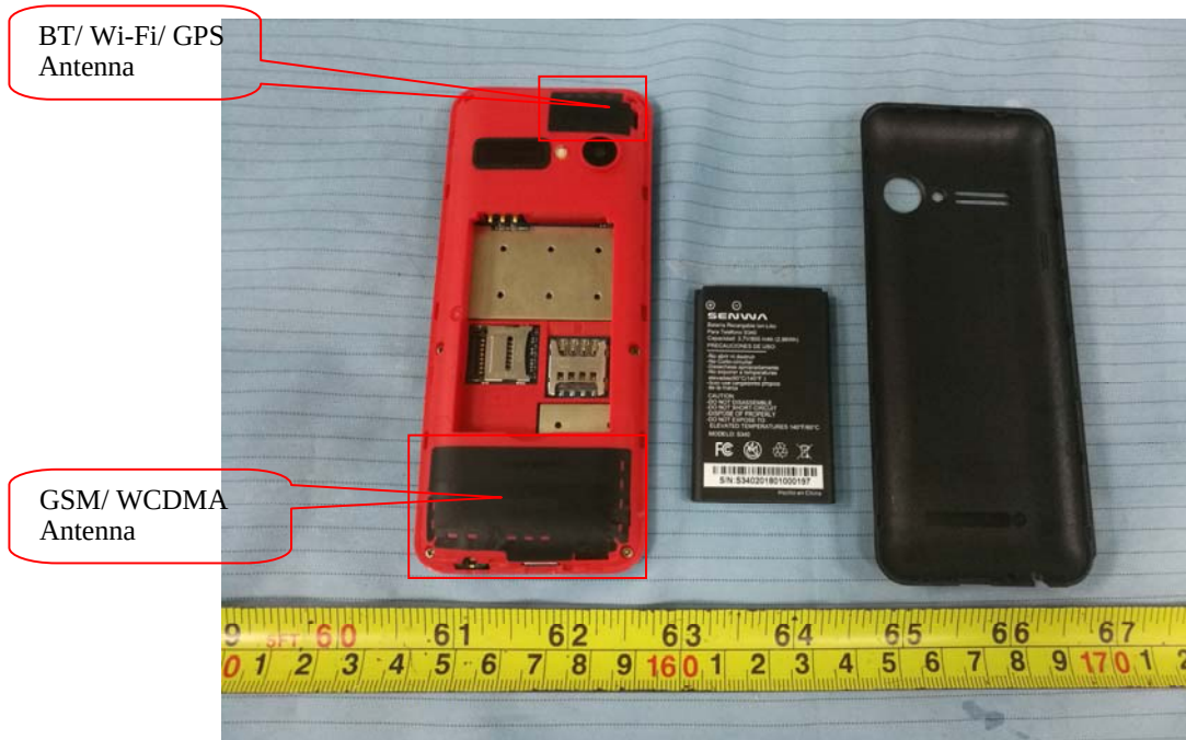
EUT – Cover off View 1
