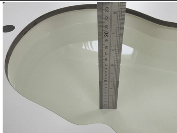
Liquid depth in the head phantom (2450MHz)
