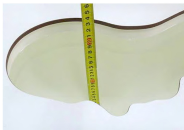
Liquid depth in the head phantom (835MHz)
