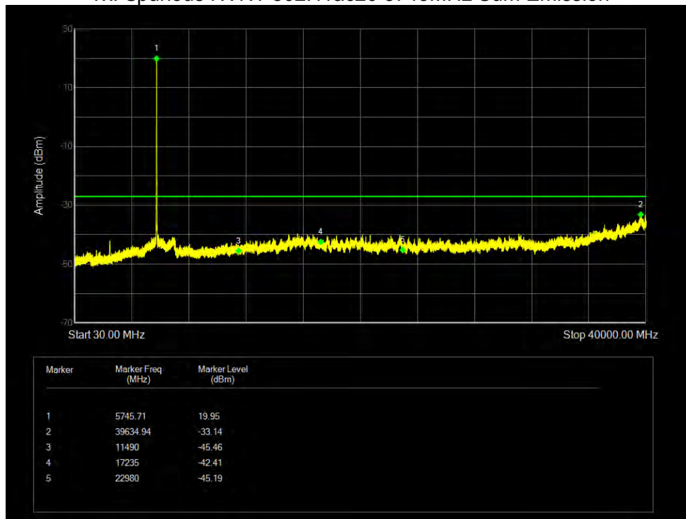
Tx. Spurious NVNT 802.11ac20 5745MHz Sum Emission
