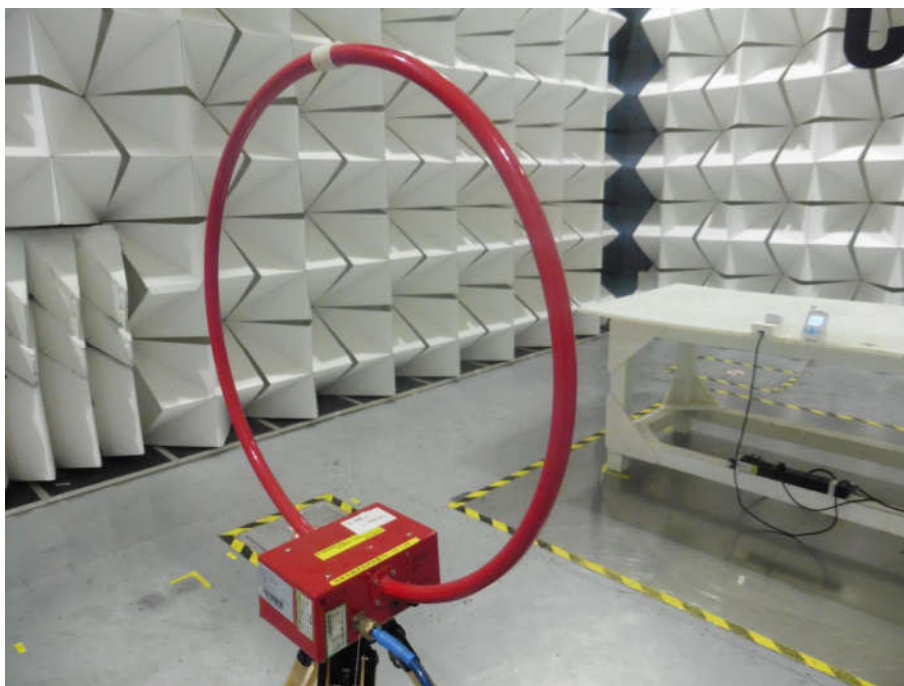
Radiated spurious emission Test Setup for adapter 2(Below 30MHz)
