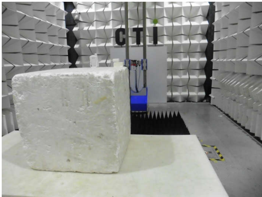
Radiated spurious emission Test Setup for adapter 1(Above 1GHz)
