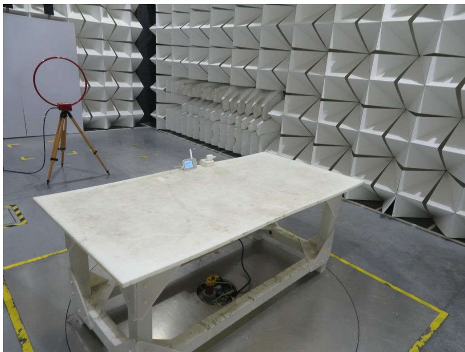
Radiated spurious emission Test Setup-3(Below 30MHz)
