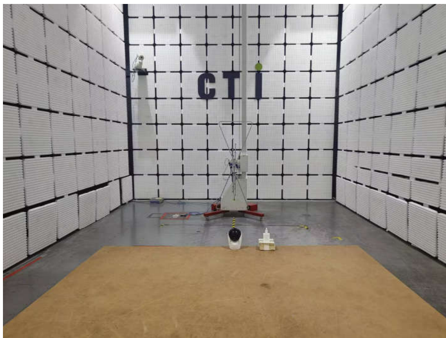
Radiated spurious emission Test Setup-1(Below 1GHz)
