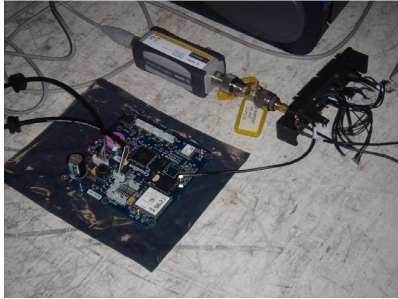
Peak Power Test Setup
