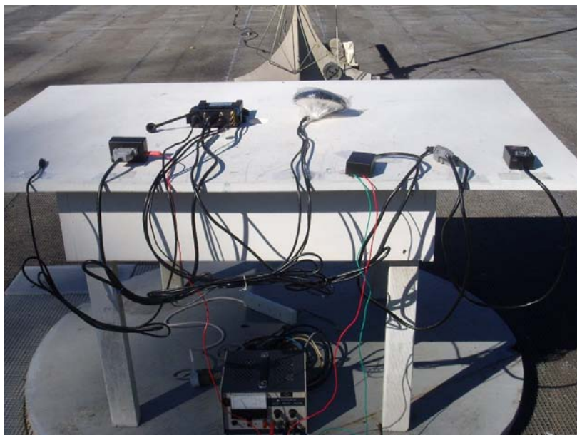
Radiated Disturbance Test Setup (Below 1GHz for MA600 Antenna) – View 1
