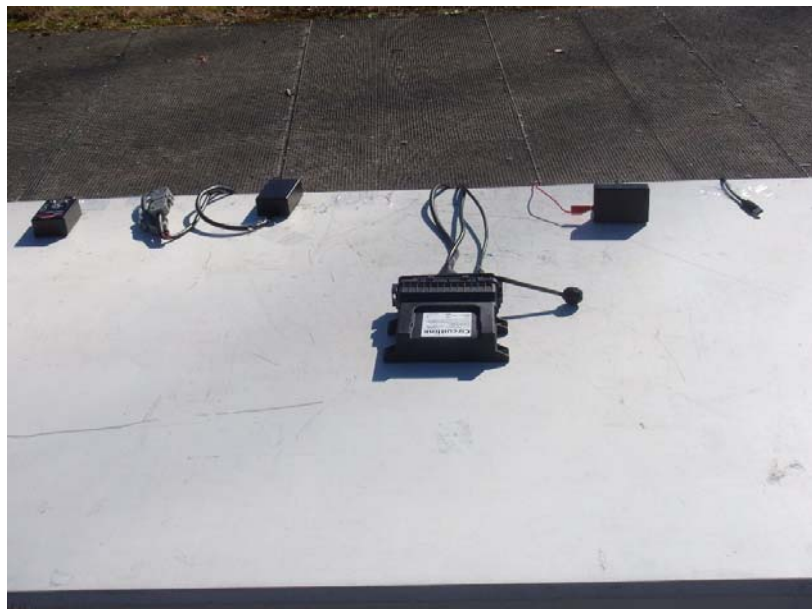
Radiated Disturbance Test Setup (Below 1GHz for Stub Antenna) – View 2
