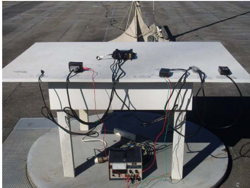
Radiated Disturbance Test Setup (Below 1GHz for Stub Antenna) – View 1
