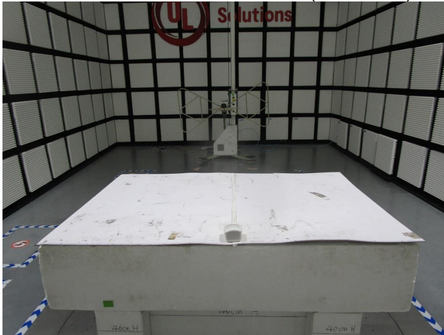
RADIATED RF MEASUREMENT SETUP (Below 30MHz)
