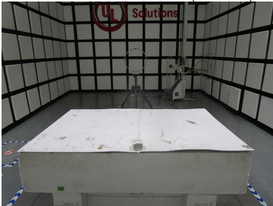
RADIATED RF MEASUREMENT SETUP (Below 30MHz)
